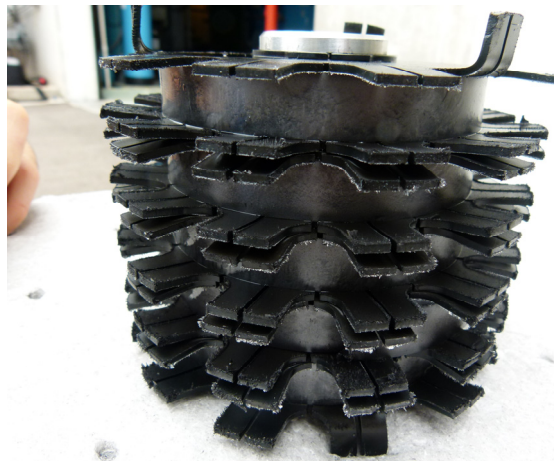
Fig. 2 Metal debris (reflective flakes) trapped in the magnetic filter
