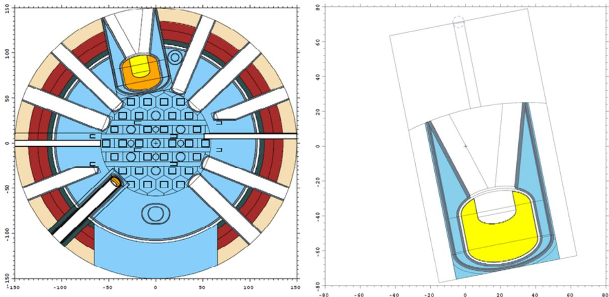
Figure 2. MCNP models of the NBSR core (left) and the LD<sub>2</sub> cold source (right). The surface source generated from the core calculation provides the starting neutrons for the CNS performance calculations (note the DXTRAN sphere, top right in the center).
