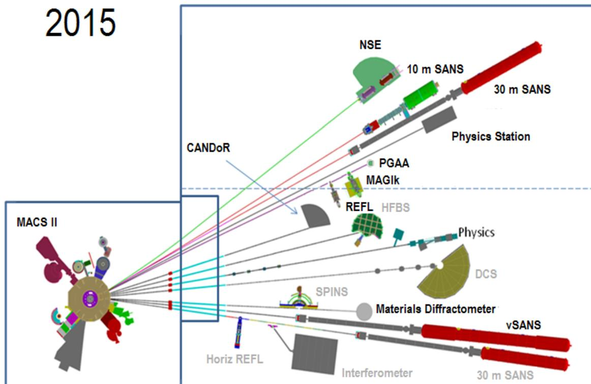
Figure 1. Anticipated layout of cold neutron instruments at the NCNR upon completion of the Expansion Project funded by the national American Competitiveness Initiative. The new guide hall, above the dotted line, nearly doubles the area of the cold neutron facility, and increases the number of guides from 7 to 12.
