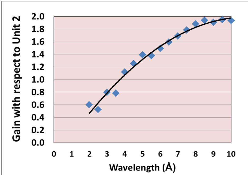
Figure 3. Anticipated gains of the LD<sub>2</sub> cold source with respect to the existing LH<sub>2</sub> source.
