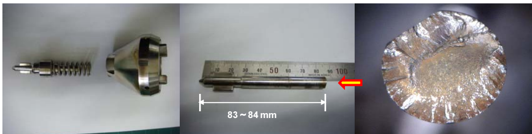
Fig. 5. Failed rod tip of the 11M-19K out-pile capsule
