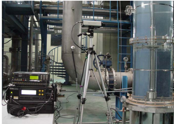
Fig. 4. Measuring the vibration of a capsule installed in the single channel out-pile test loop
