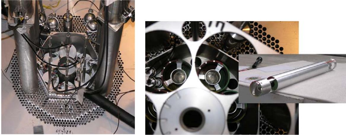
Figure 1. Cross section of the AMMON reference core. Left: bird eye-view; Right: zoom on the central part and of one JHR fuel element
