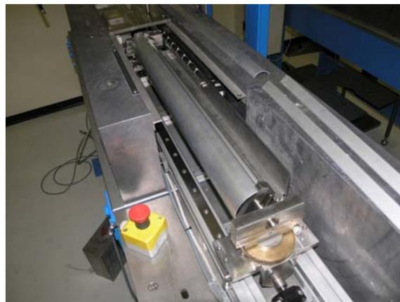
Figure 2. Top view of the  $\gamma$ -scanning bench for curved plate axial and azimuthal measurements
