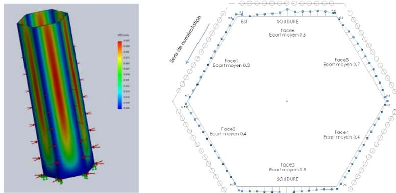
Figure 5. Central chimney deformation due to water pressure (left) - Average shape vs theoretical shape (0.3 to 0.7mm discrepancy) on the central cask (right)
