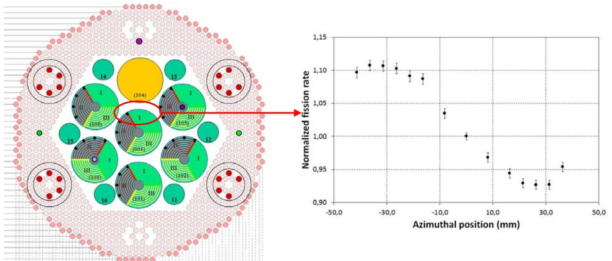
Figure 4. Azimuthal fission profile on external plate of the central assembly, in the “Beryllium periphery” configuration. Left : configuration – Right : fission rate profile
