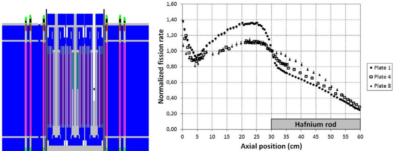
Figure 3 Axial fission profile on plates 1 (inner), 4 (mid) and 8 (outer) of the central assembly, in the “1/2 hafnium” configuration. In this particular configuration, an hafnium rod is inserted in the central assembly.
