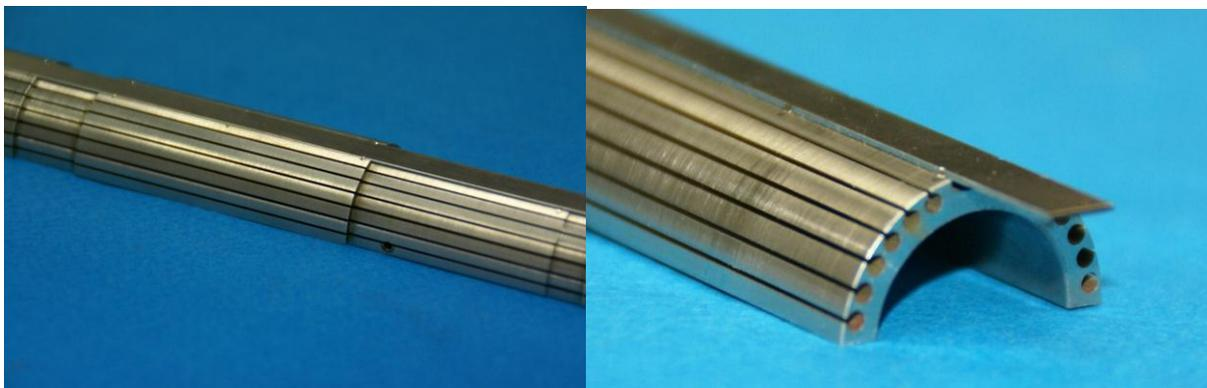
*Fig. 5: The half shell which contains thermocouples during processing*
