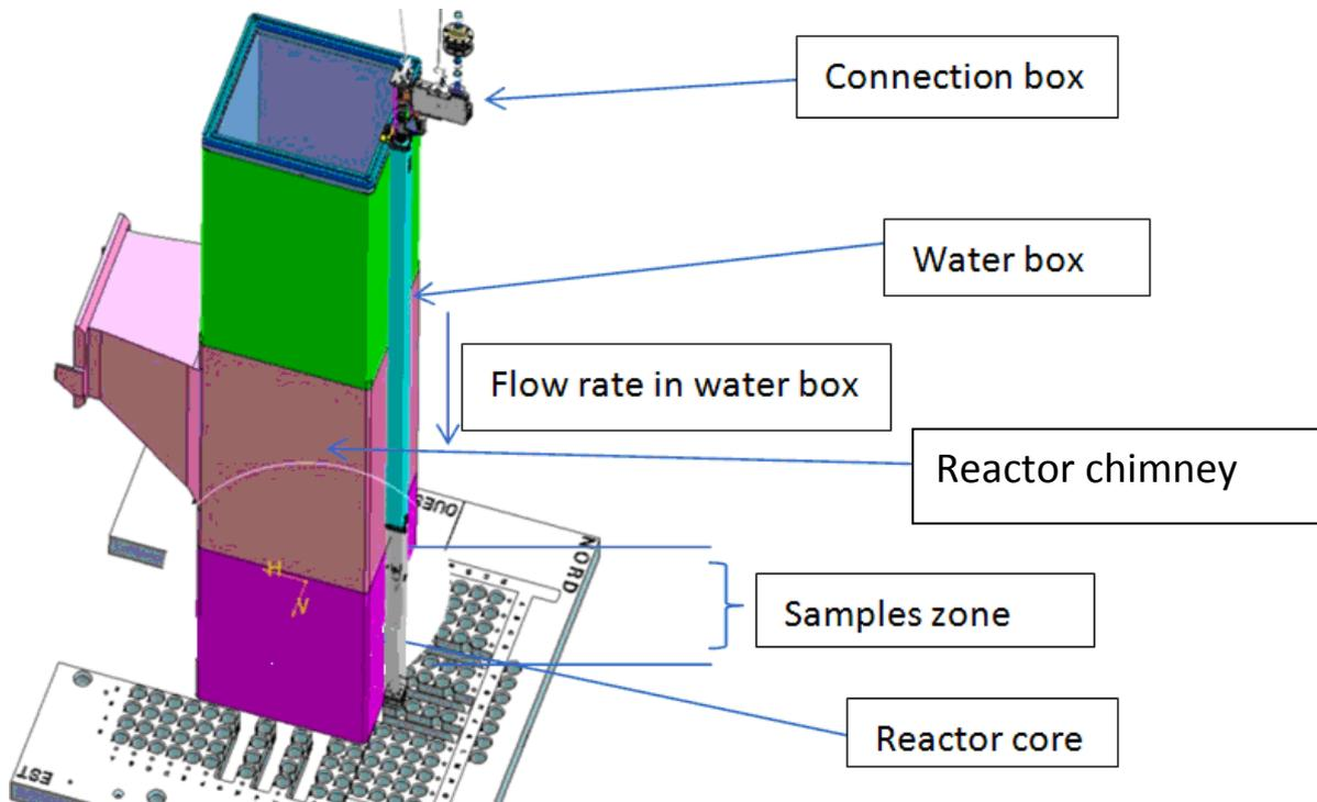
Fig. 3: Device in the water box on the reactor out-core
