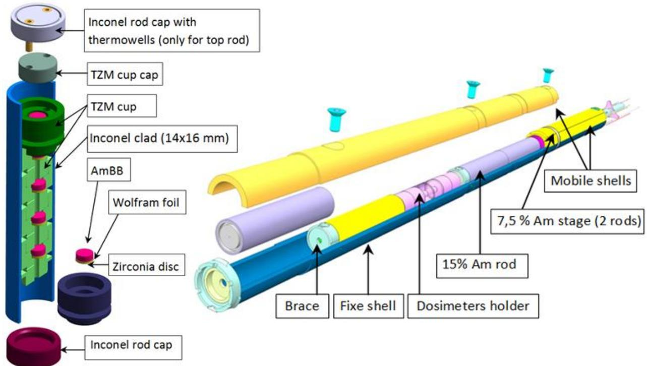
Fig. 1: Needle details and shell of the sample holder with needles and thermal separator
