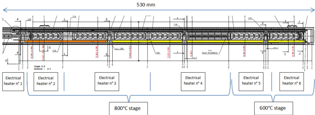
Fig. 2: Bottom of the sample holder in the safety double barriers PHAETON furnace
