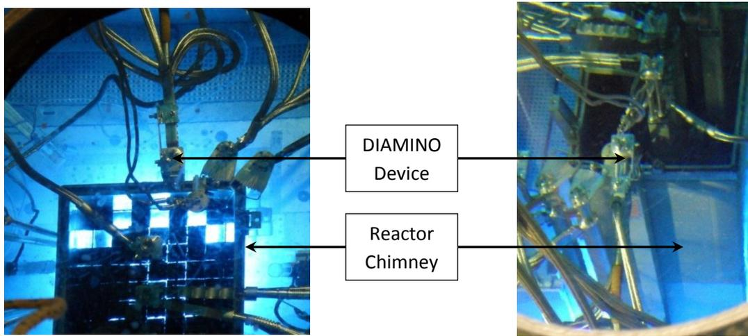
Fig. 4: Device on the reactor out-core
