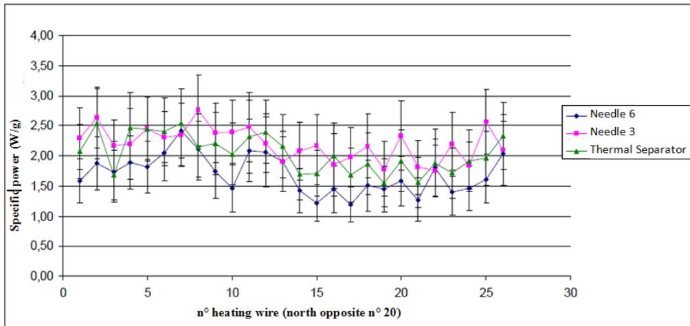
Fig. 7: Azimuthal distribution of gamma heating in heater wires at the level of needles 3 and 6 and thermal separator ( $\times 1.42$  W/g)
