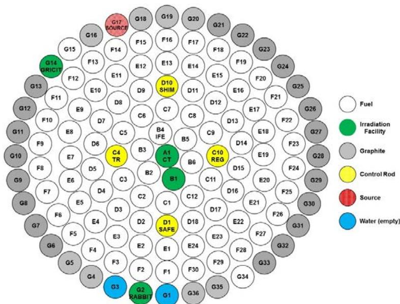
*Figure 1 – Diagram of Original LEU Core Configuration*
