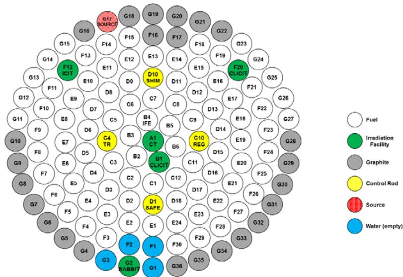
Figure 2 – Diagram of New LEU Core Configuration
