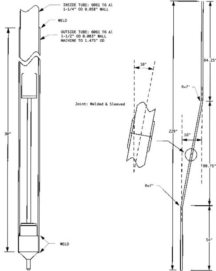
Figure 3 – Cross Section of In-Core Irradiation Tube
