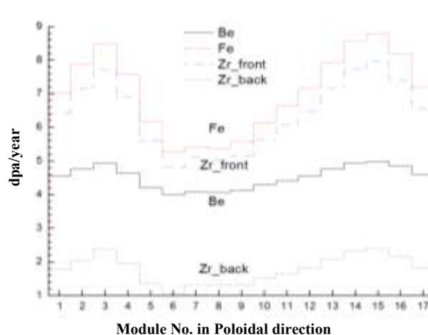
*Fig. 5 First wall dpa distribution around poloidal direction*
