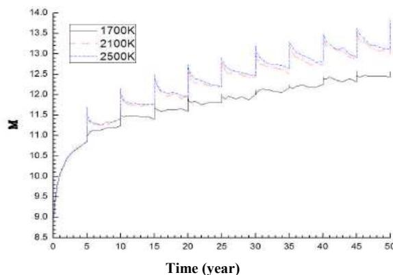
Fig. 3 *M vs. time under three pyro-reprocessing temperature*
