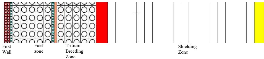
Fig. 2 Radial cross section of the fuel module
