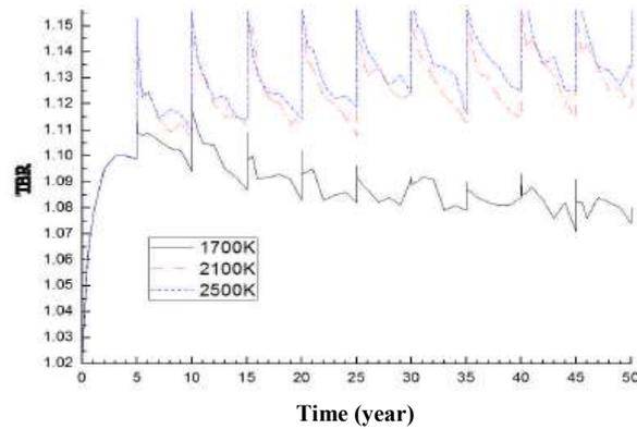
Fig. 4 TBR vs. Time under three pyro-reprocessing temperature
