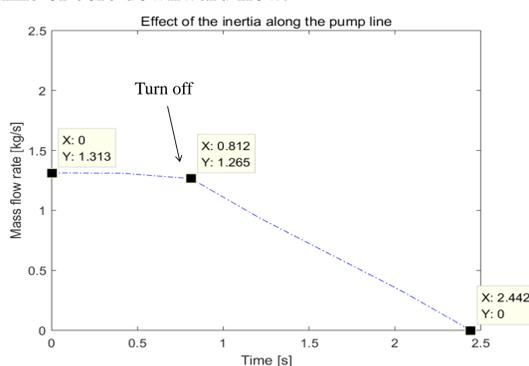
FIG. 5. Mass flow rate of the Pump (1.8 m, 3/4 inch)
