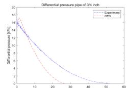
FIG. 5. Differential pressure at the DPP (1.8 m, 3/4 inch DPP)
