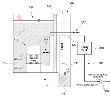
FIG. 1. Conceptual drawings of PRHRS
