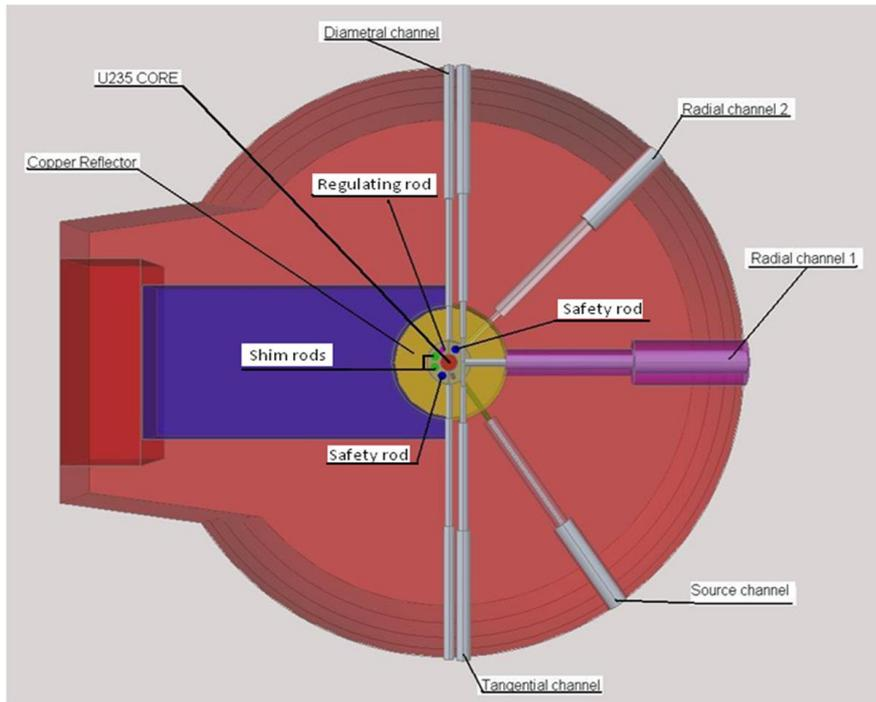
Figure 2. TAPIRO horizontal section.
