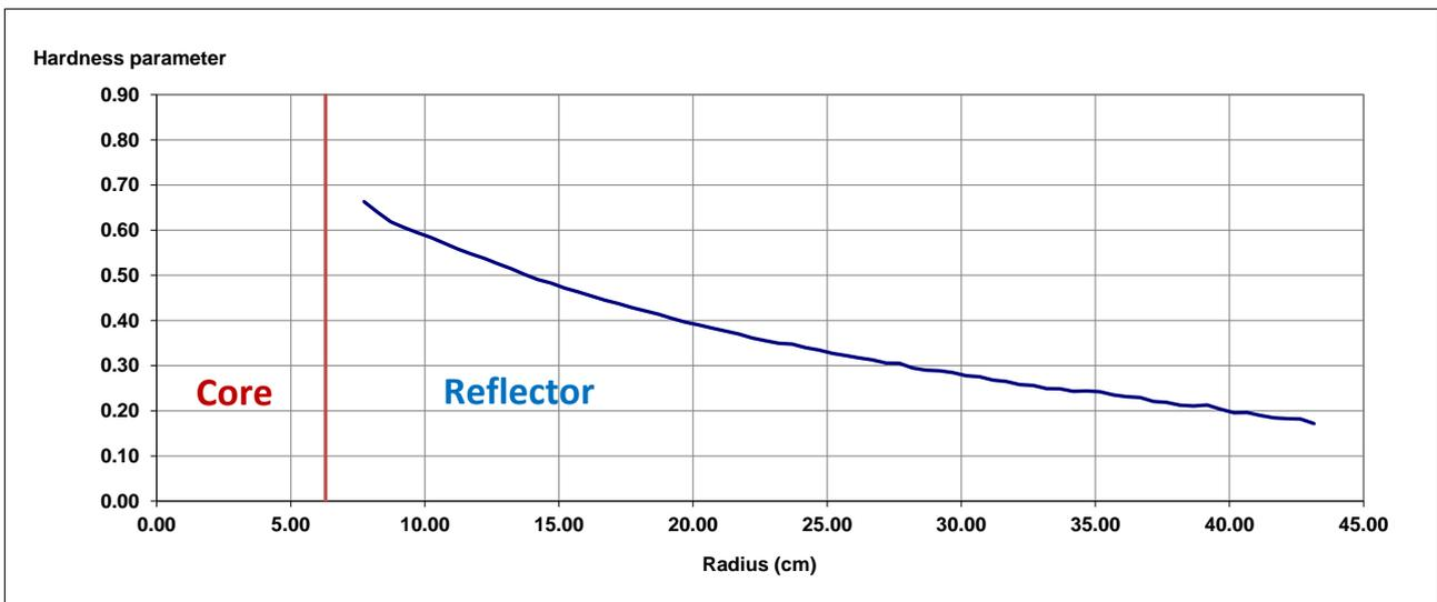
Figure 8. Hardness parameter radial behavior for TAPIRO radial 1 channel.
