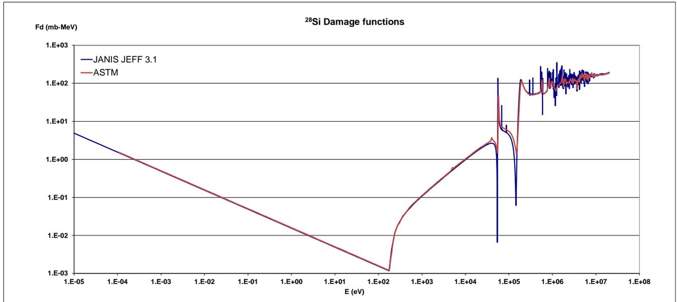
Figure 1. Comparison between damage KERMA functions for  $^{28}\text{Si}$  provided in [5] and JEFF 3.1.
