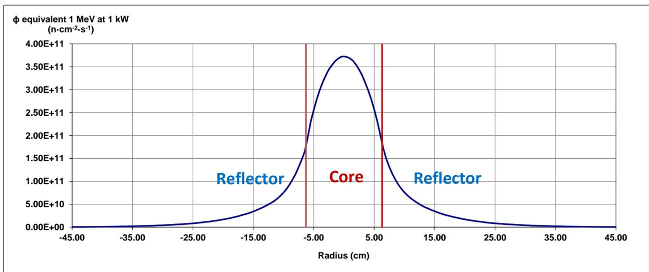
Figure 5. Equivalent 1 MeV flux radial behavior for TAPIRO diametral channel at 1 kW power.
