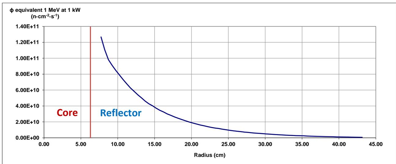
Figure 6. Equivalent 1 MeV flux radial behavior for TAPIRO radial 1 channel at 1 kW power.
