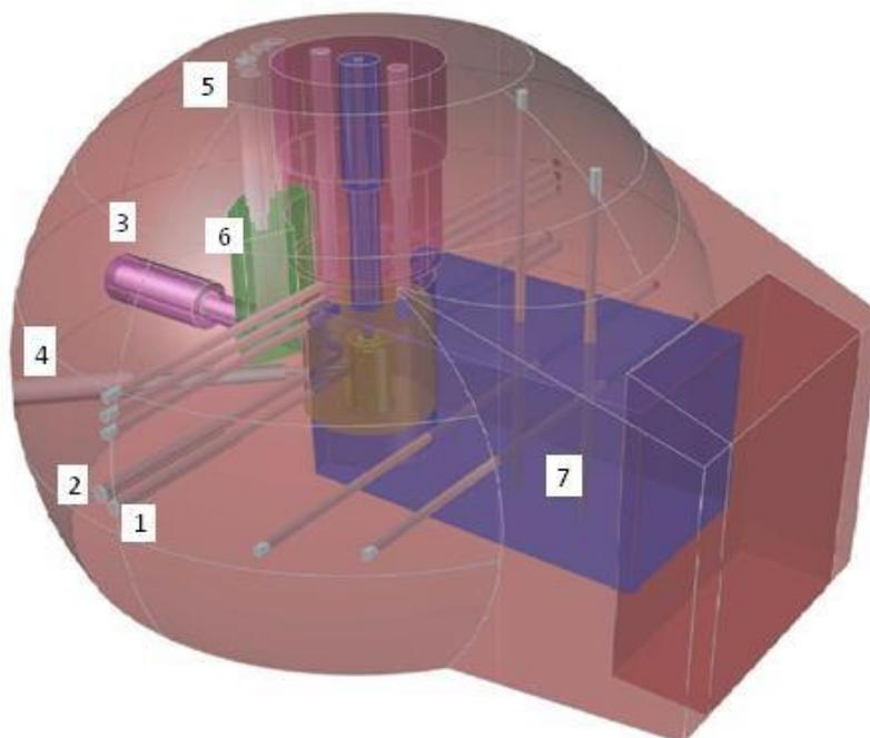
Figure 3. TAPIRO Irradiation facilities: 1) diametral channel; 2) tangential channel; 3) radial channel 1; 4) radial channel 2; 5) detector channels; 6) paraffin; 7) thermal column.
