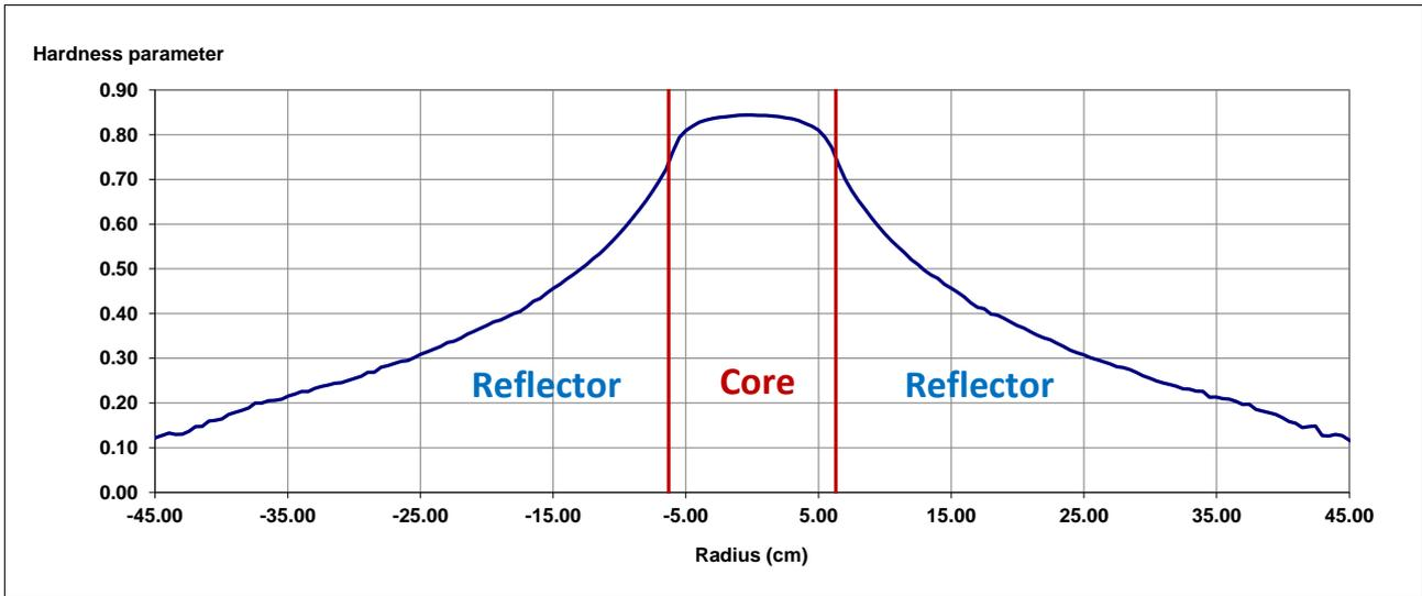
Figure 7. Hardness parameter radial behavior for TAPIRO diametral channel.
