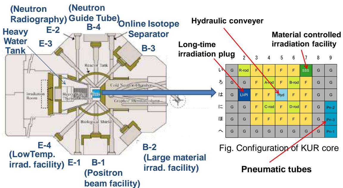
Fig. 1 KUR core and experimental facilities configuration
