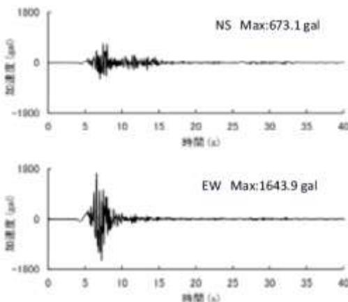
Fig.3 Horizontal Accelerations of the Basis Ground Motion for KUR Seismic Evaluation
