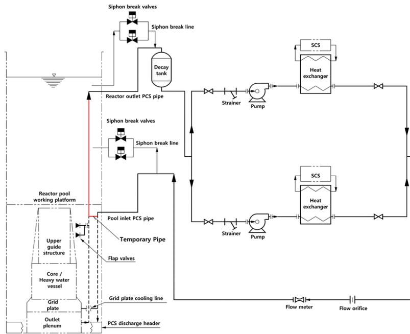
FIG. 2. Primary Cooling System for Closed Flushing
