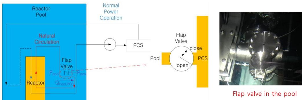
FIG. 6. Flap Valve installed in the Pool
