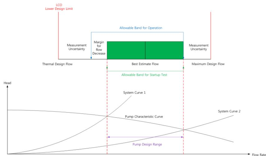
FIG. 4. PCS Pump curve and PCS flow design
