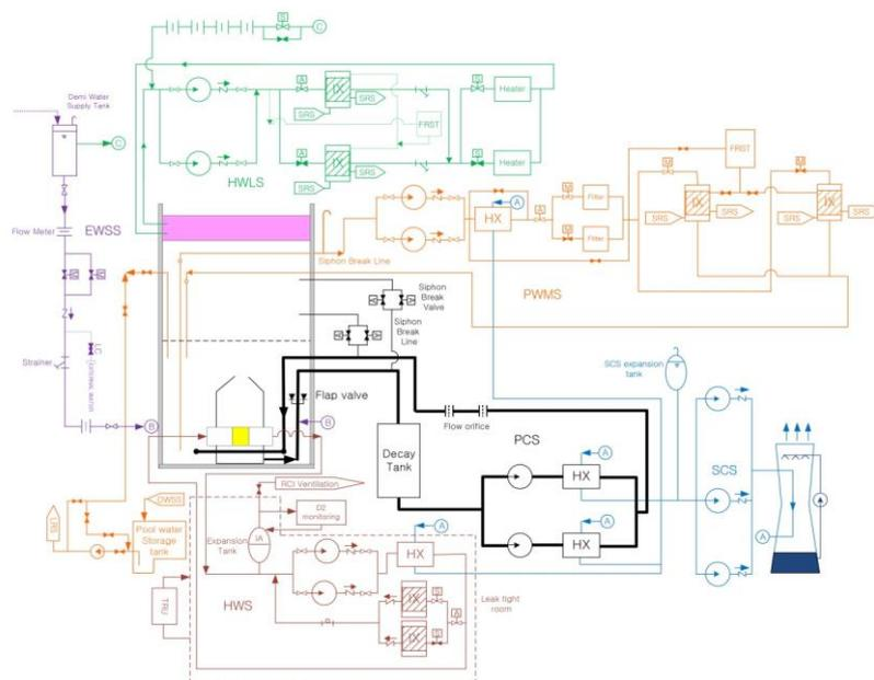
FIG. 1. Flow Diagram of Reactor Cooling and Connected Systems (Open Flushing)
