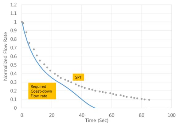
FIG. 5. Coast-Down Flow using Flywheel of PCS Pump
