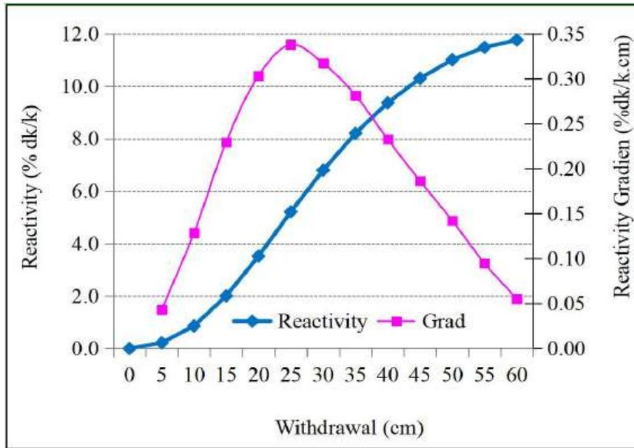
Fig.6. S-Curve control rod worth and its gradient
