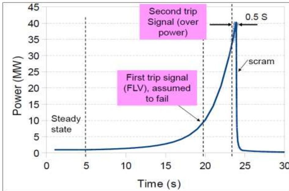
Fig.7. Event sequence of reactivity insertion accident
