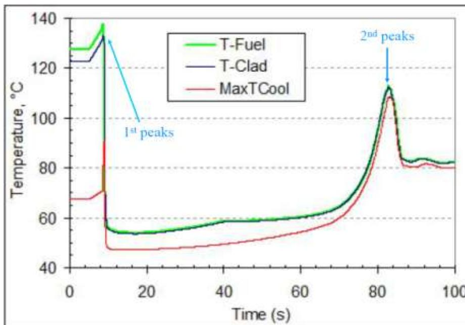
Fig. 2. Fuel, clad and hottest coolant temperature during LOFA
