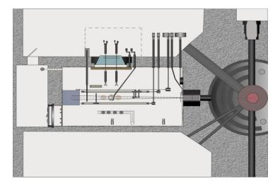
**Neutron radiography cell** 7.1 m (length) × 4.1 m (width) × 2.9 m (height)
