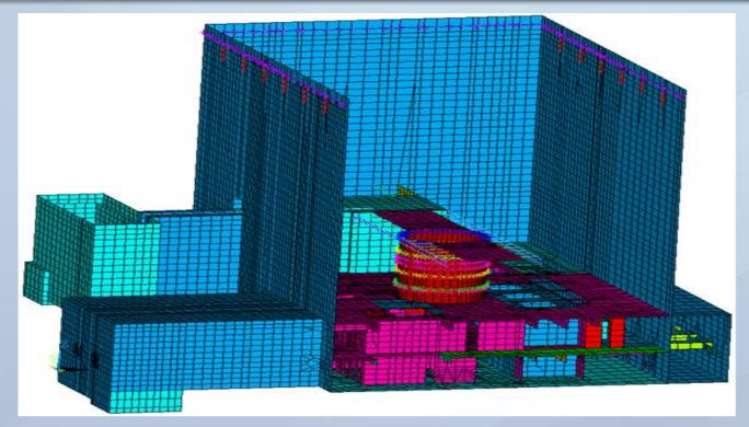
3 Dimensional Finite Element Model of Dhruva Reactor Some portion of the walls is not meeting the present requirements. Retrofitting to strengthen the wall being done
