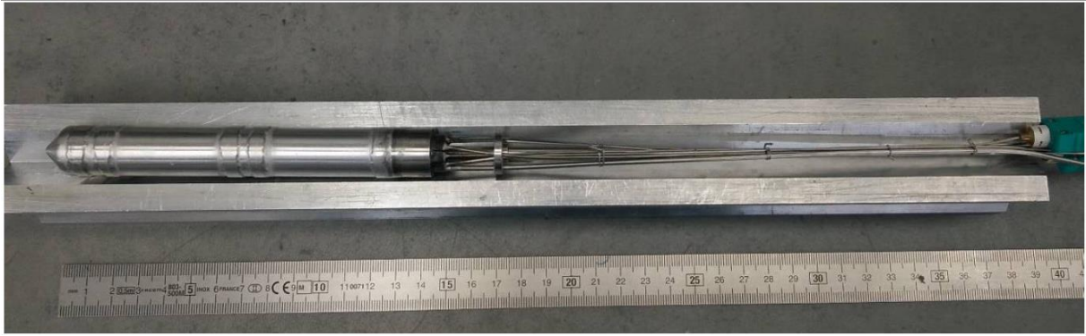
Figure 6: Calorimeter mock-up before and after assembly
