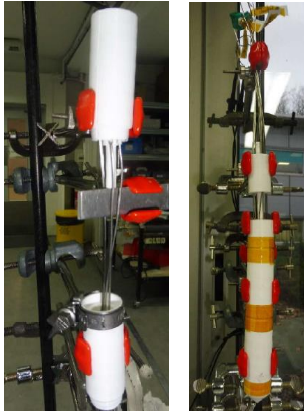
Figure 8: Assembly of the 3D model printed calorimeter
