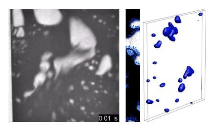
FOV = 70 mm square, 130  $\mu$ m/pixel, L/D~150,  $\Phi_{peak}$ =3.25×10<sup>6</sup> cm<sup>-2</sup>s<sup>-1</sup>/frame
