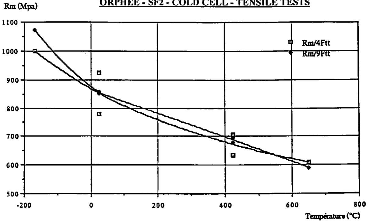
Figure 6 : Ultimate strenght. Comparison between face 4F and 9F (heat treated samples).
