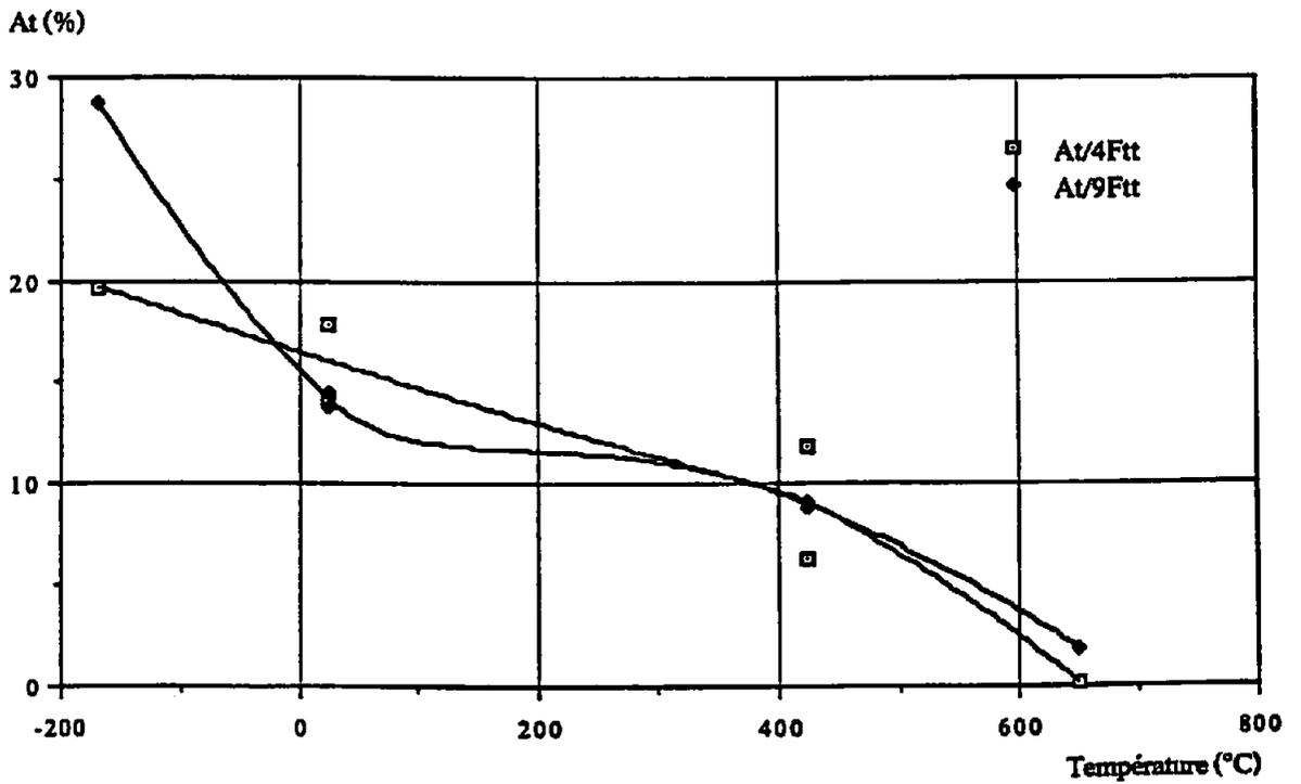
Figure 7 : Total elongation. Comparison between face 4F and 9F (heat treated samples).
