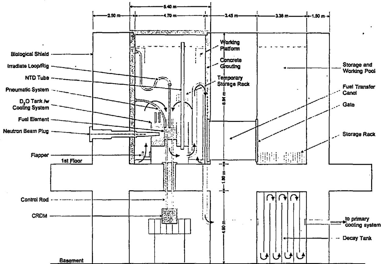
**Fig. 1 A vertical cross section view of TRR- II**
