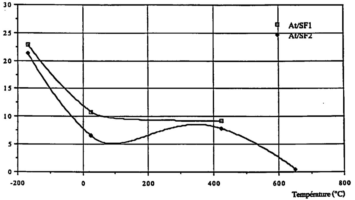
Figure 10 : Total elongation. Comparison between SF1 and SF2 (non heat treated samples).
