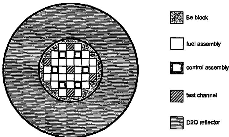
Figure 1. TRR-II core configuration
