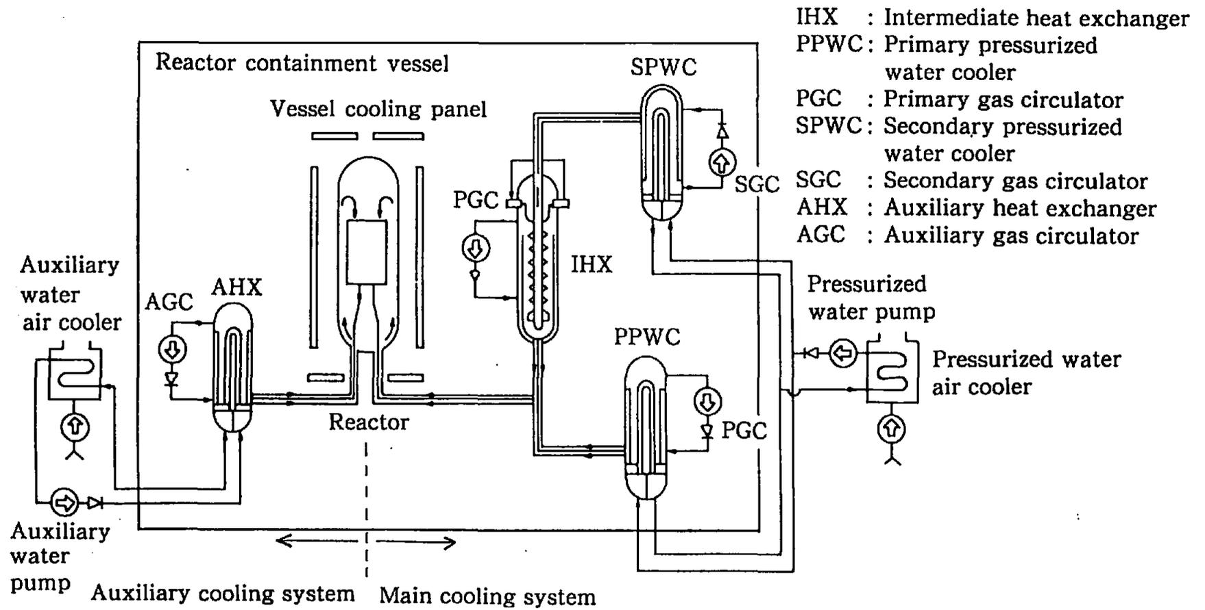
Fig.3 Cooling system in the HTTR.
