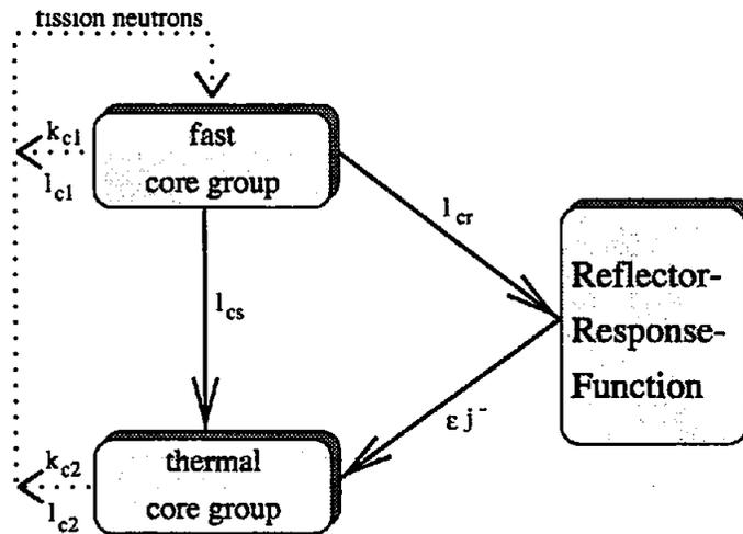
**Figure 2:** Schematical illustration of the two points-two groups kinetics model with the continuous Reflector Response Function  $G(\tau)$ . The arrows represent the neutronic coupling; the  $k$ -symbols designate coupling efficiencies, the  $l$ -symbols stand for transfer delays.
