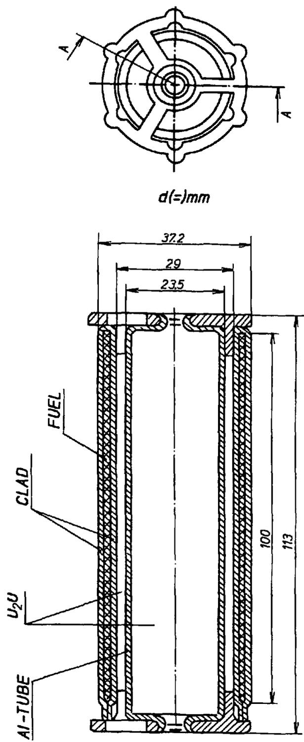
Figure 2. Cross section of the research reactor RA fuel element
