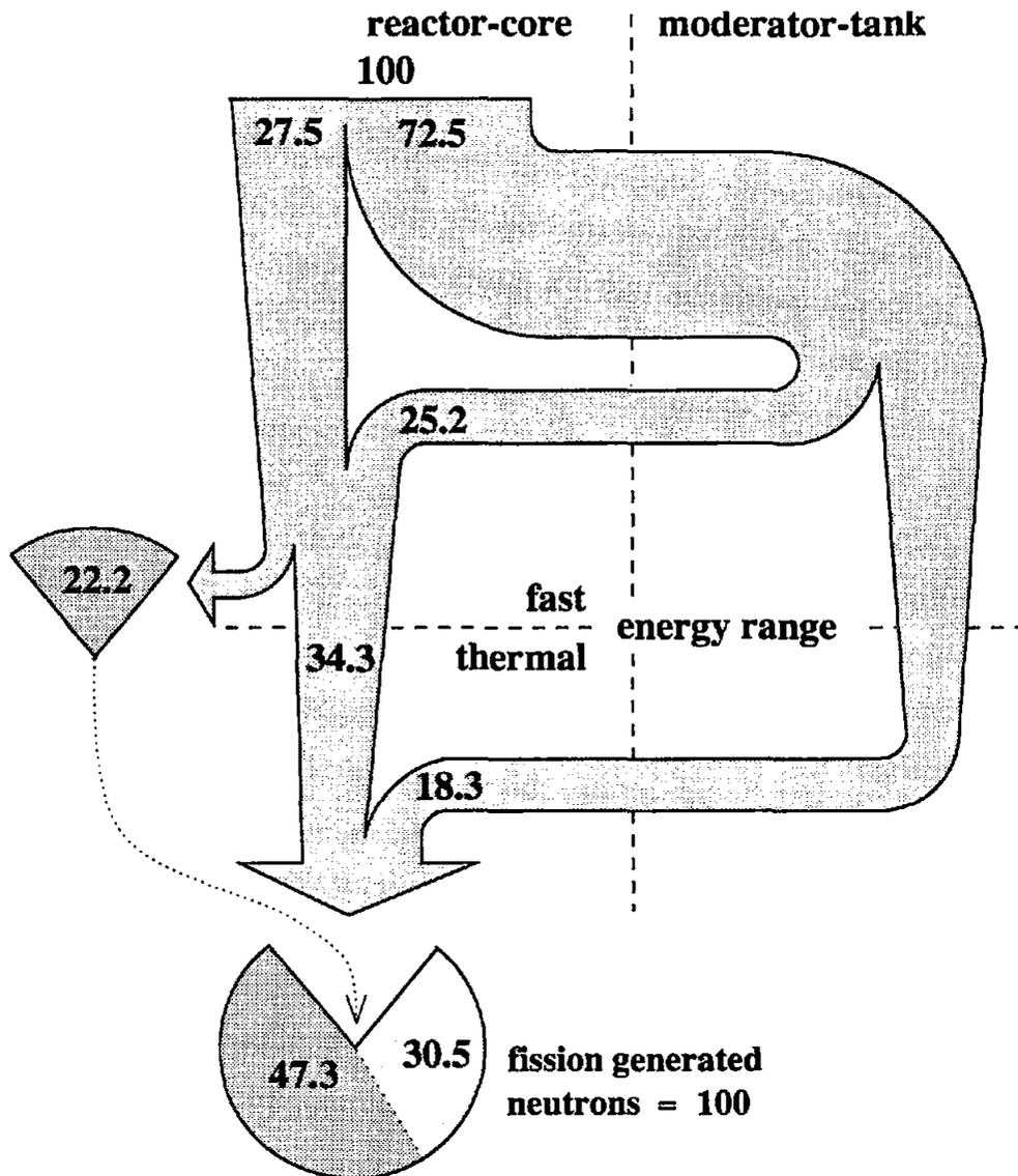
**Figure 1:** Schematical depiction of the neutron life cycle in the KKE7. Decreasing bar-width symbolizes absorption- and leakage-losses, circle sections represent the contributions to the production of the next generation of fission neutrons; the thermal energy limit is 0.6 eV. The part “reactor-core” comprises the control rod region. Therefore, a part of the 34.3 neutrons moderated in this path, serv for reactor control, i.e. are absorbed in the absorber section of the control rod.
