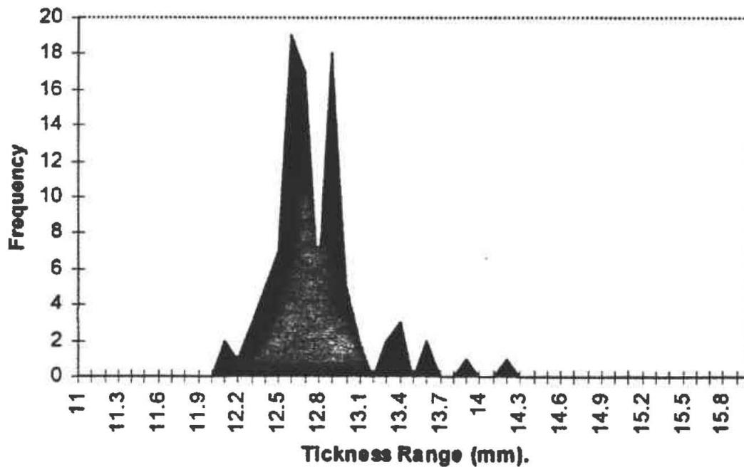
Figure 3. Histogram of RAT Wall Thickness Values
