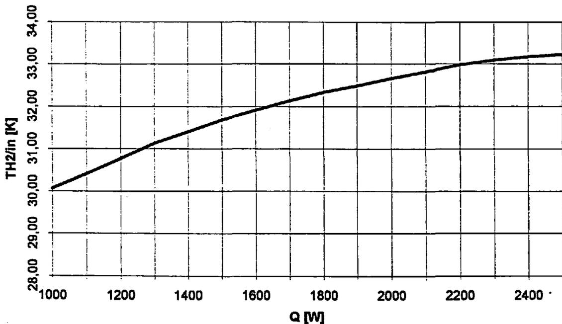
**Fig. 4 Calculated heat exchanger temperatures for various heat absorbed power ( $T_{\text{out}}=21.5\text{K}$ ,  $p=15\text{bar}$ )**
