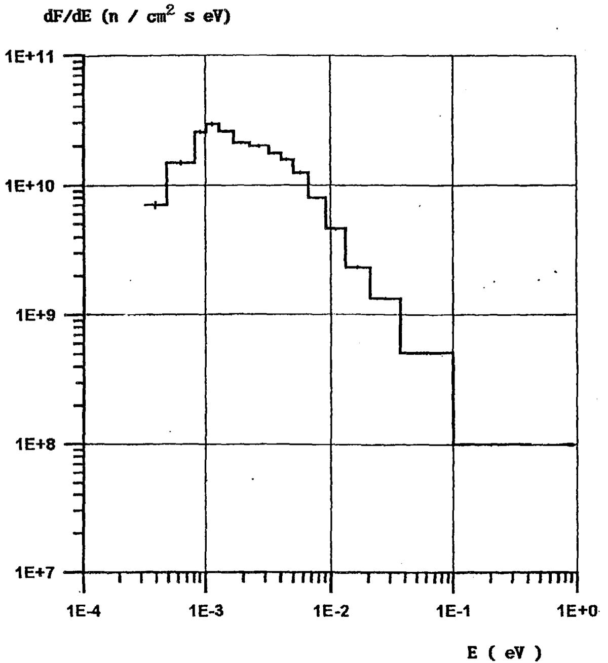
Fig.4. Neutron spectrum inside cold neutron source
