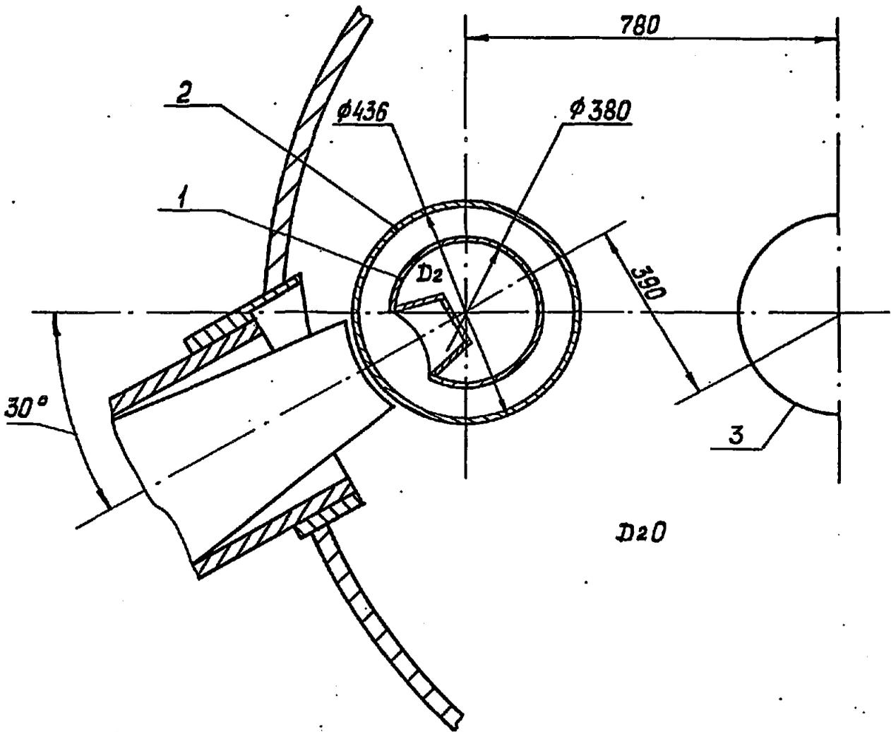
**Fig.2. Layout of CNS in the heavy water reflector**
