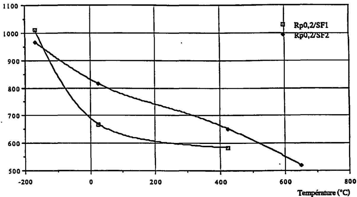
Figure 8 : Yield strenght evolution. Comparison between SF1 and SF2 (non heat treated samples).
