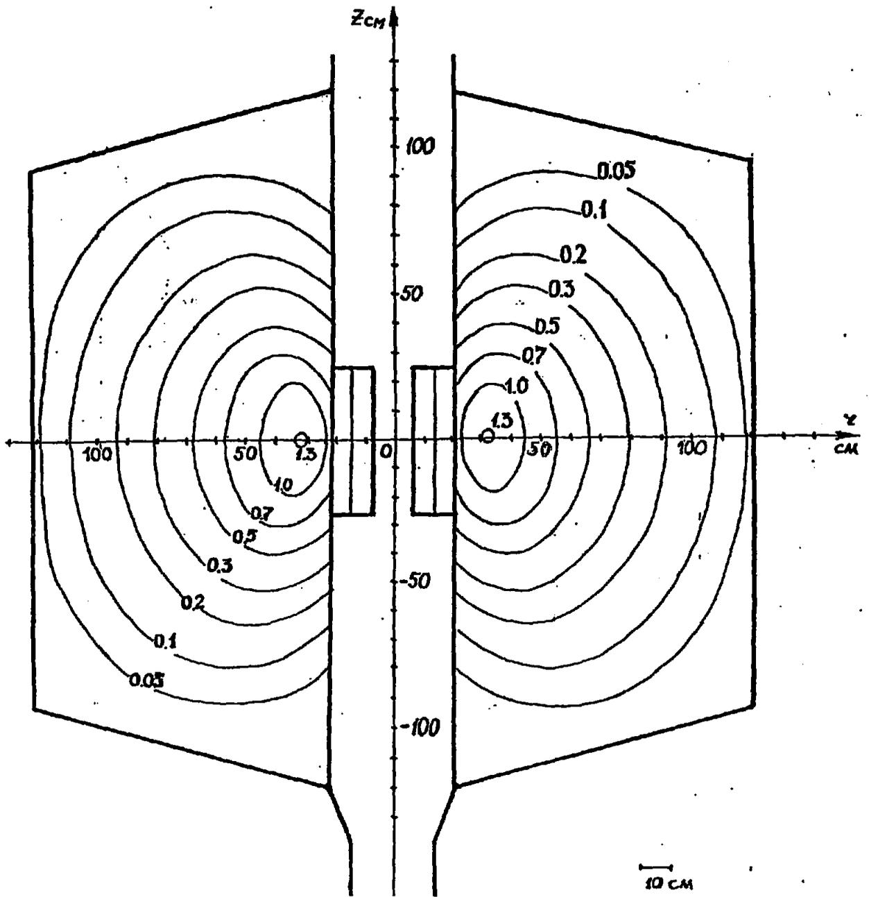
Fig.6. Thermal neutron flux distribution,  $10^9$  n/cm<sup>2</sup>s
