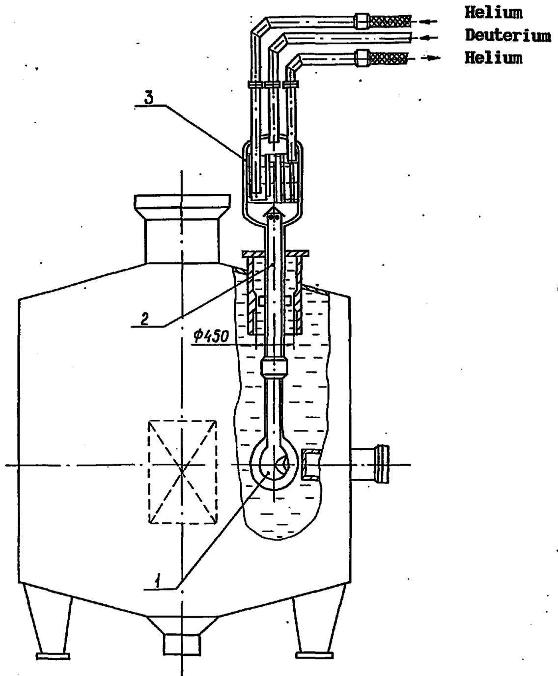
**Fig.1. Layout of CNS at the reactor facility**
