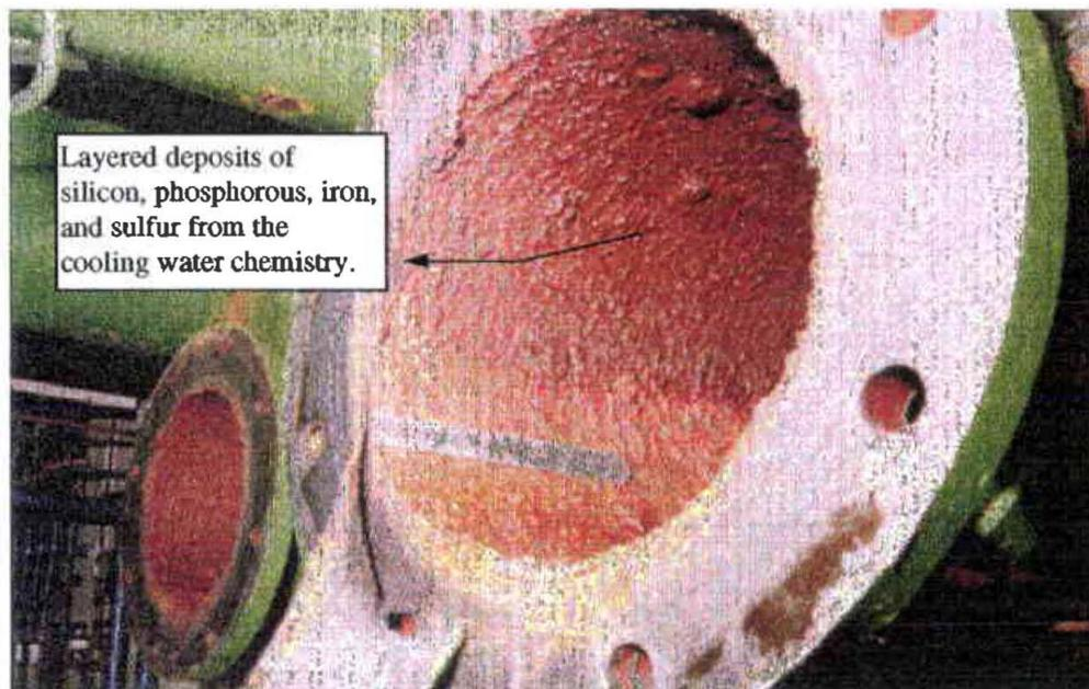
Figure 8. Corrosion Deposits inside the Old SCWC Pipework
