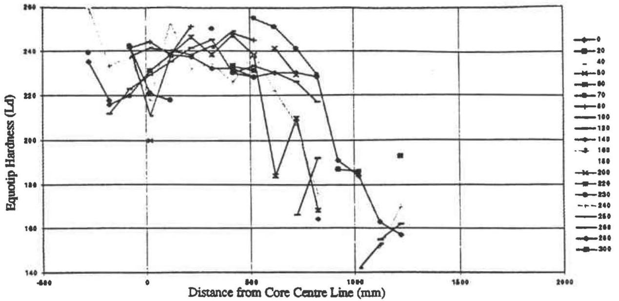
Figure 2. RAT Wall Hardness Profile at Various Angles
