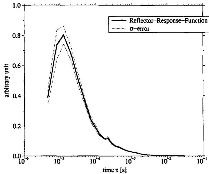
**Figure 3:** Linear-log plot the the Reflector Response Function  $G(\tau)$  of the FRM-II, without experimental installations in the moderator tank. The function has been determined by Monte Carlo calculations and is normalized to
