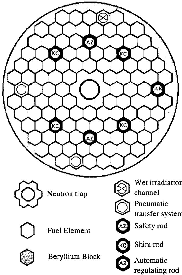
Fig. 2 WORKING CONFIGURATION OF REACTOR CORE
