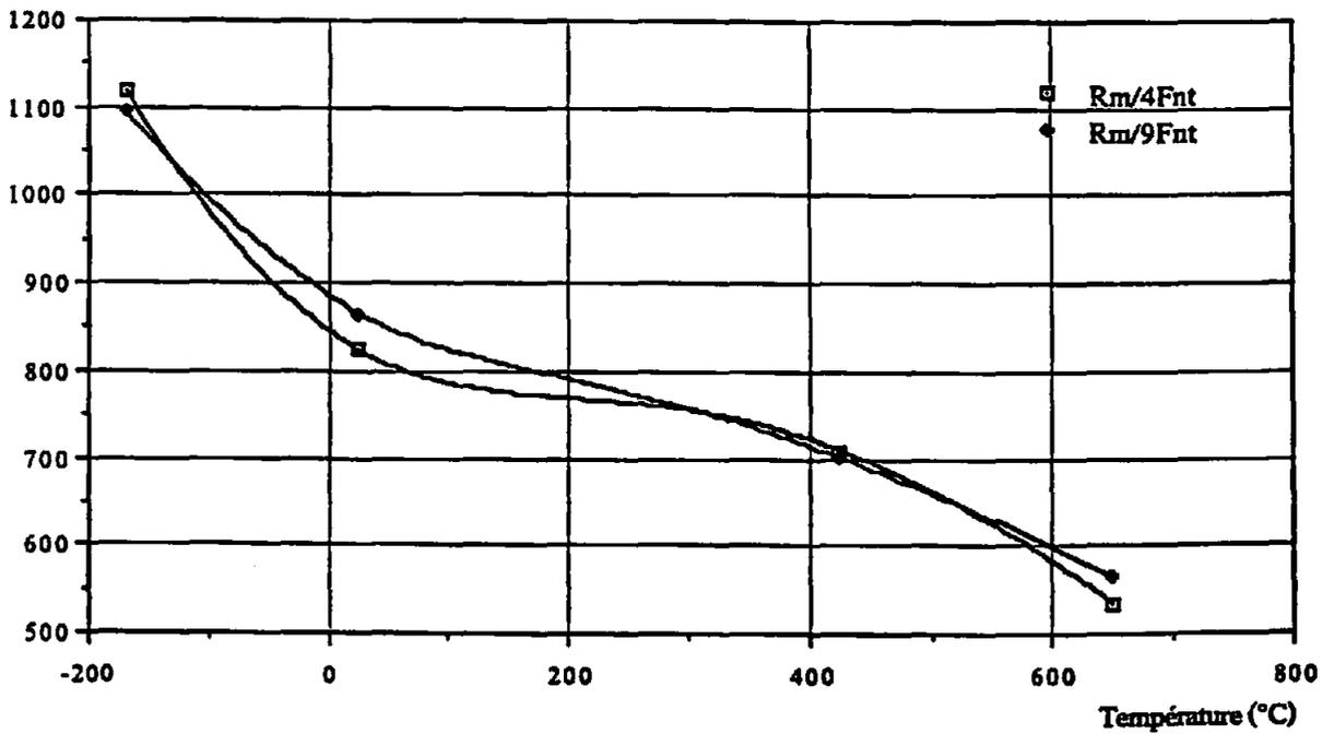
Figure 3 : Ultimate strenght evolution. Comparison between face 4F and 9F (non heat treated samples).
