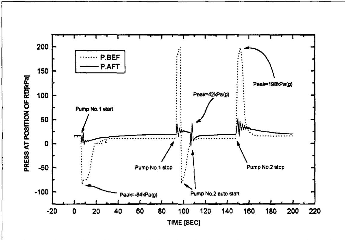
Figure 3. Pressure Transients Behaviors on RCS Pump Startup and Stop
