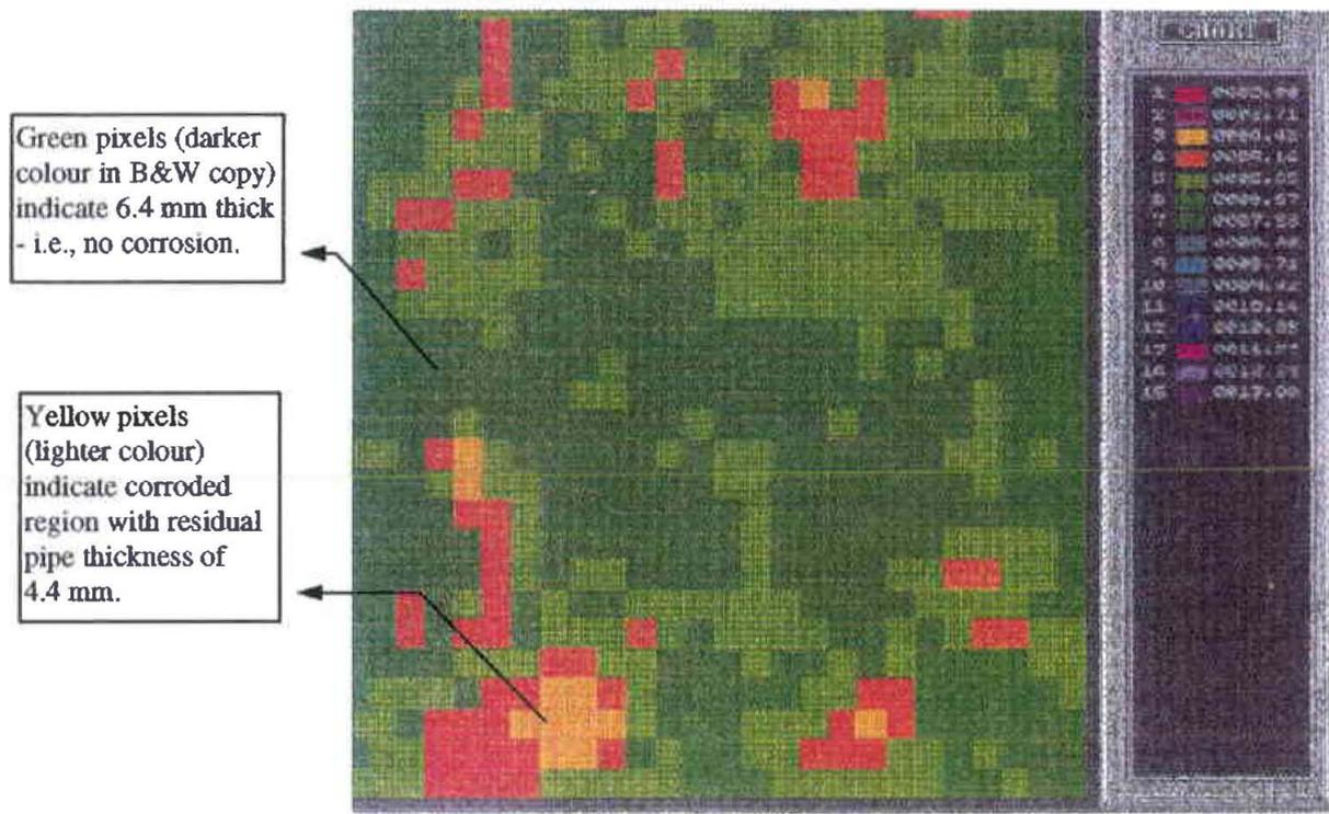
Figure 7. Micro-Map Image of the Old SCWC Pipe Thickness
