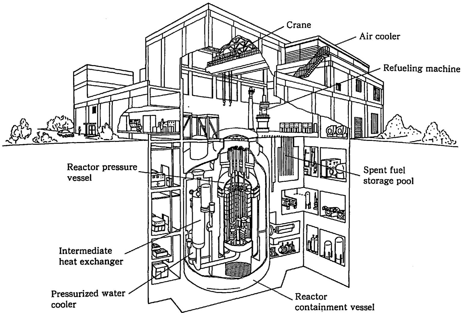
Fig.1 Bird's-eye view of the HTTR reactor building.
