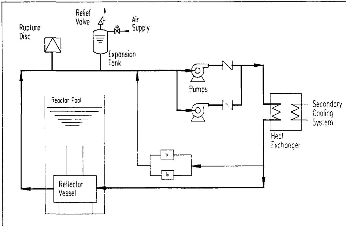
Figure 1. Flow Diagram for Reflector Cooling System
