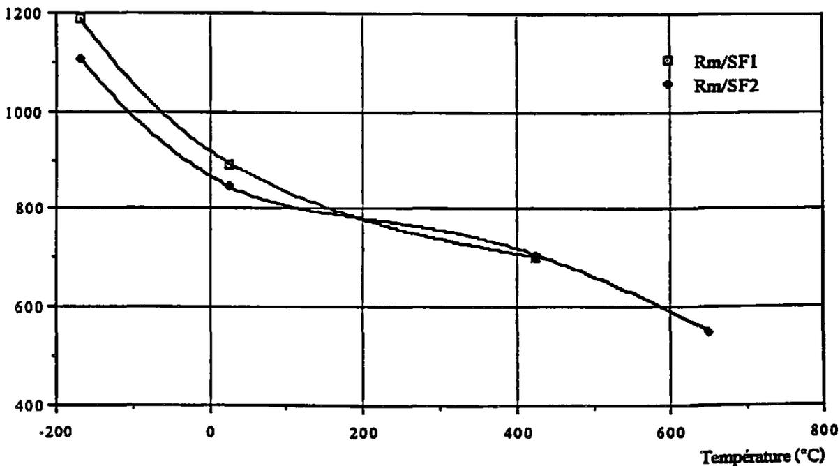
Figure 9 : Ultimate strenght evolution. Comparison between SF1 and SF2 (non heat treated samples).
