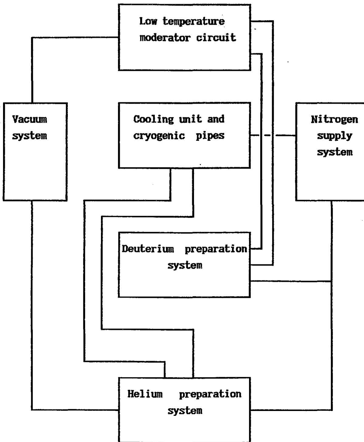
**Fig.8. Diagram of cryogenic supply**
