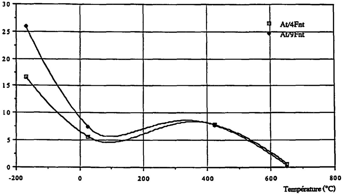
Figure 4 : Total elongation. Comparison between face 4F and 9F (non heat treated samples).
