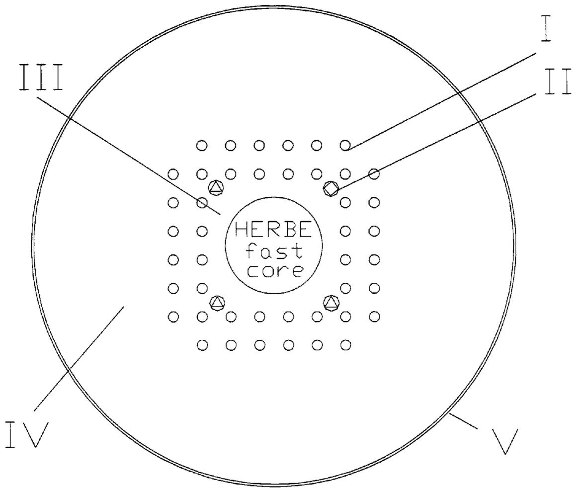
**Figure 6. Horizontal cross section of the reactor RB core with the central HERBE zone**
