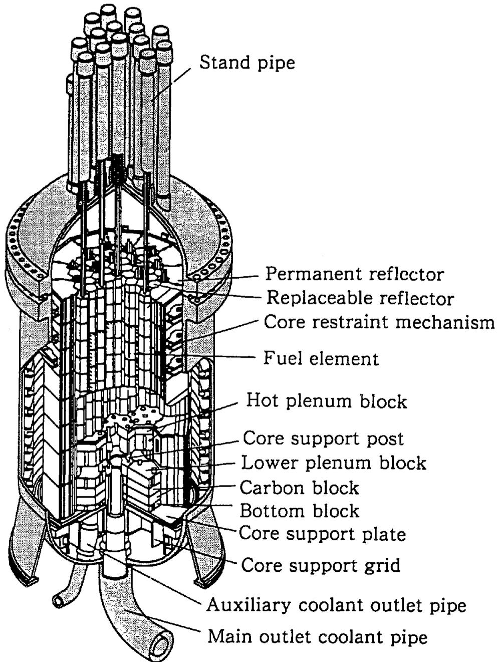
Fig.2 Bird's-eye view of the pressure vessel and the core of the HTTR.
