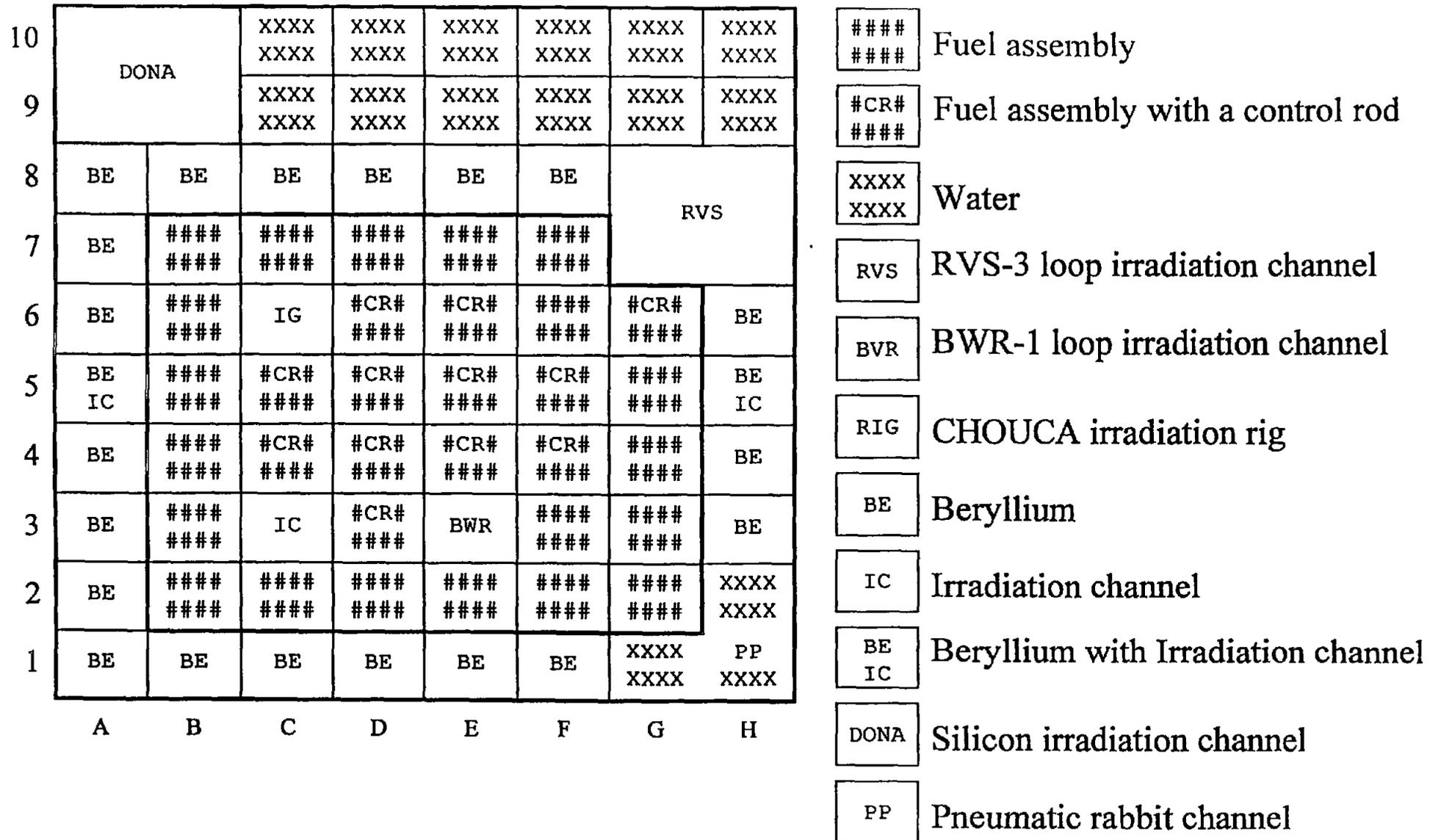
Fig. 1 LVR-15 reactor core configuration
