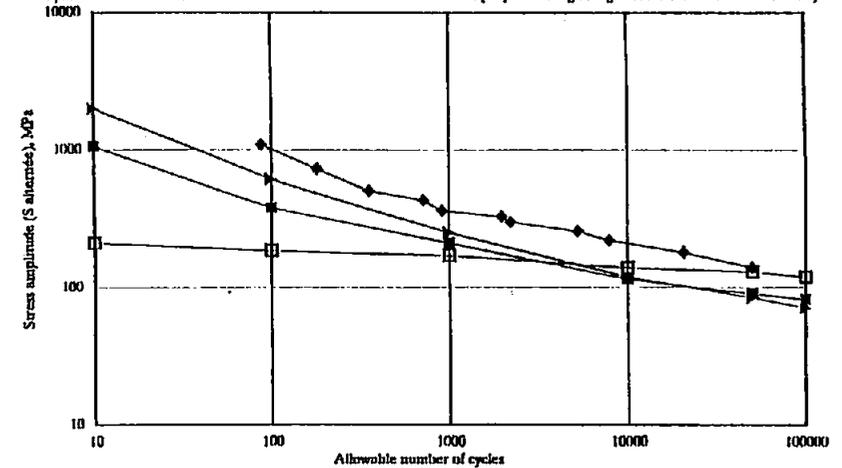
■ JAERI: tests on unirr. alloys, mainly A5052-O & A6061    ◆ ECN: Salt deduced from strain range, unir. A5154-O
