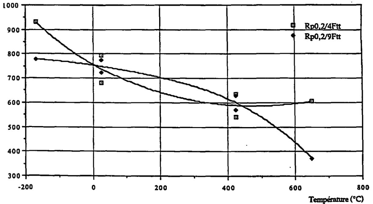
Figure 5 : Yield strenght evolution. Comparison between face 4F and 9F (heat treated samples).
