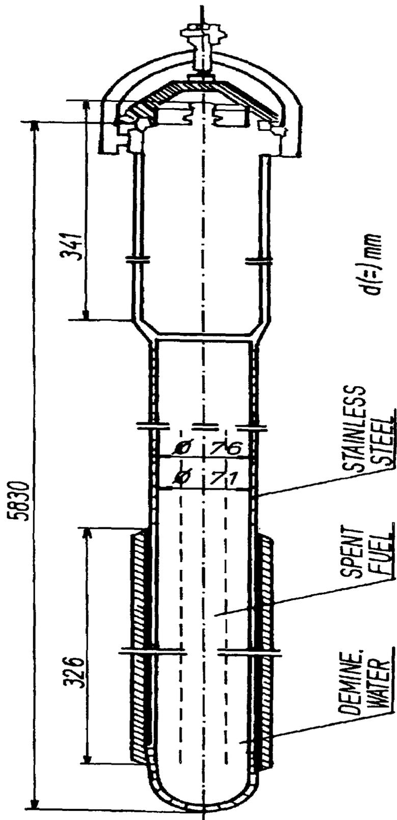
Figure 4. Stainless steel channel-type spent fuel holder
