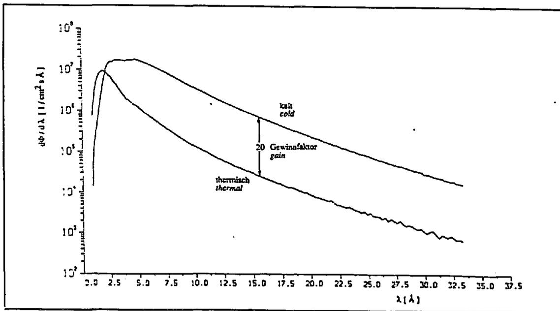
**Fig. 1 Opposition of thermal and cold neutron spectrum**
