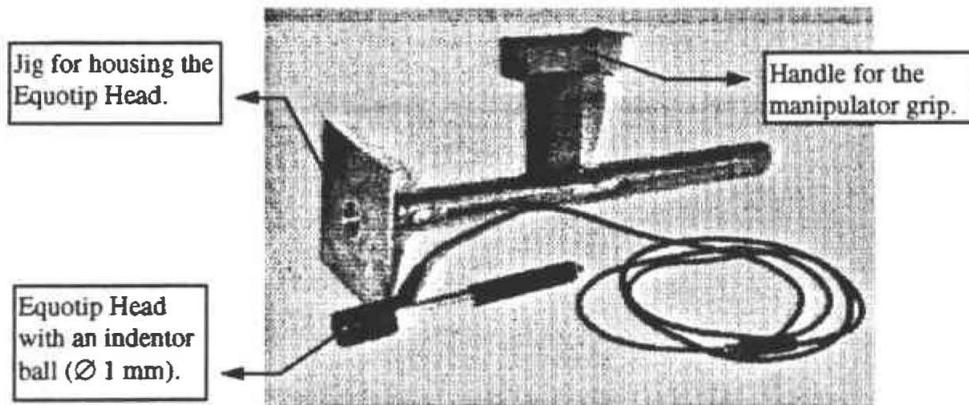
**Figure 4. Hardness Tester - 'Equotip' Head and a Jig**
