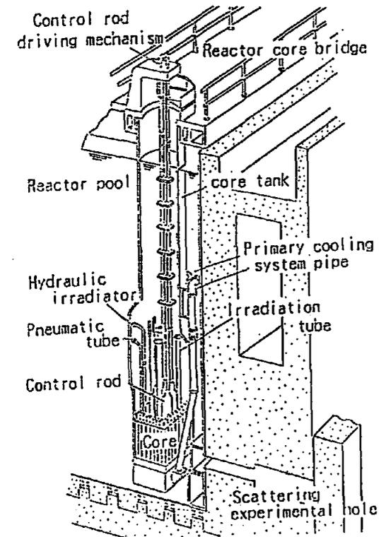
Fig. 2 A VIEW OF THE JRR-4 REACTOR
