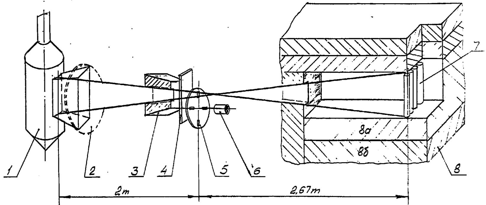
**Fig.7. Neutron time- flight installation**
