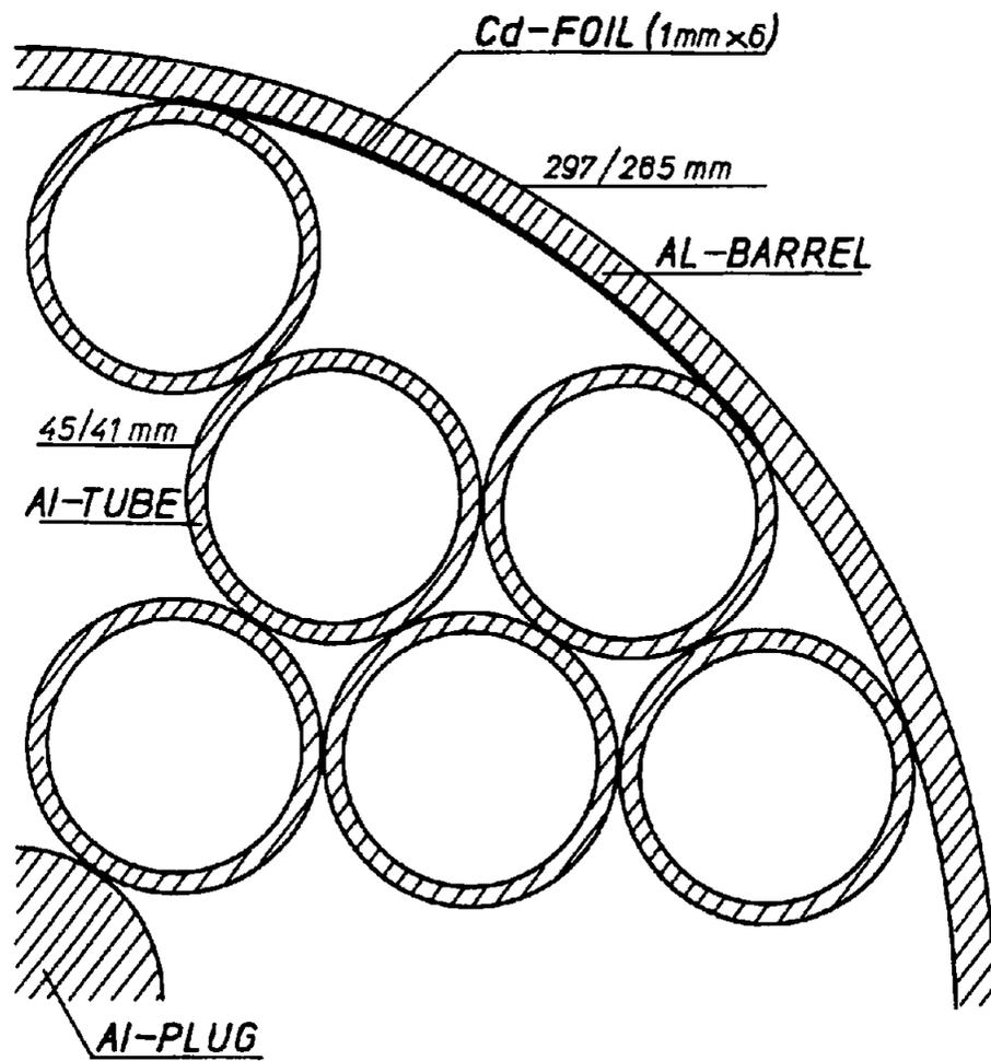
**Figure 5. Aluminium barrel with spent fuel**
