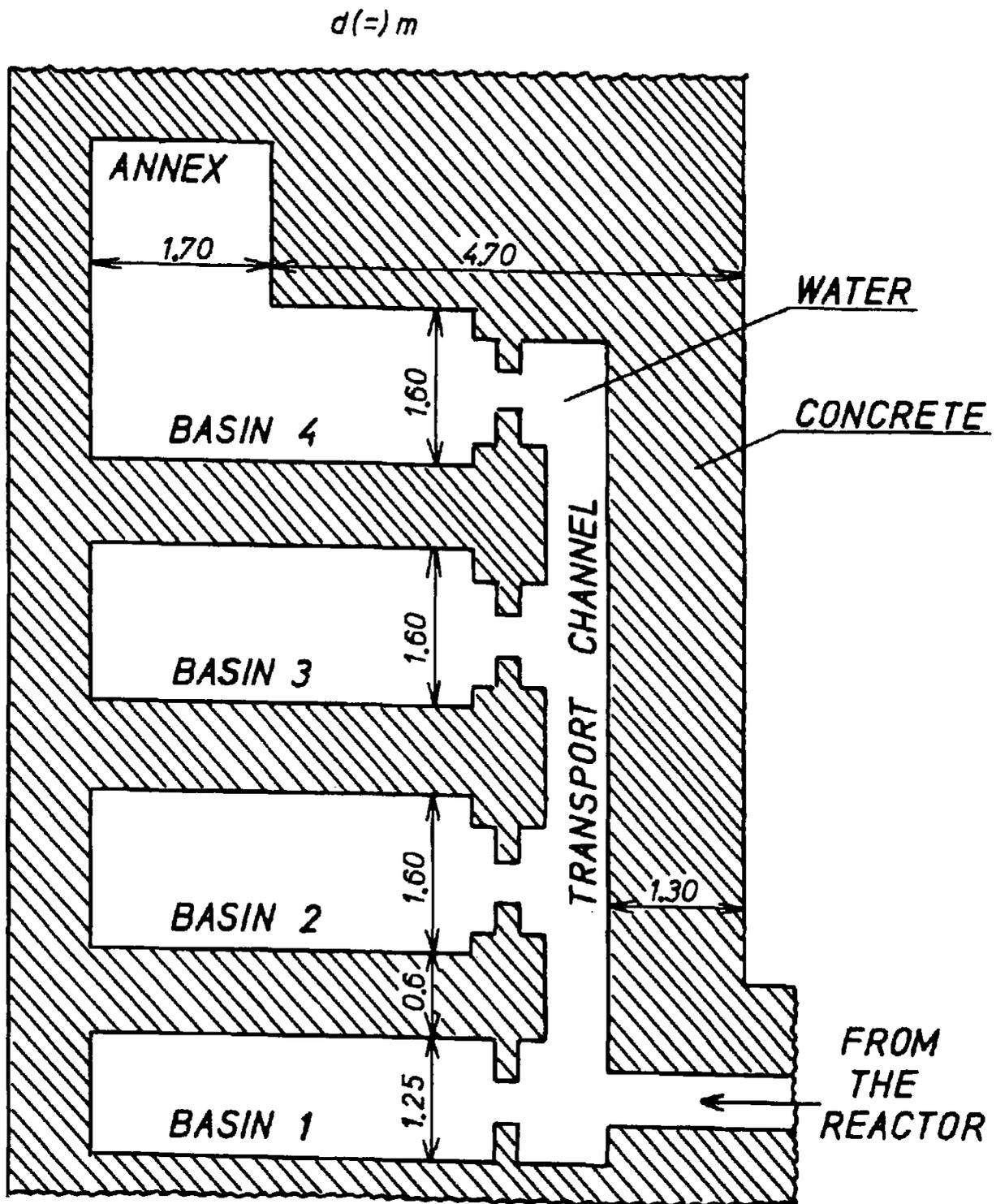
Figure 3. Scheme of the temporary spent fuel storage pool
