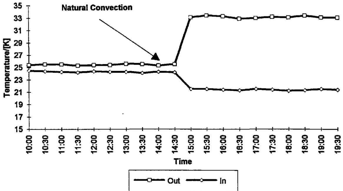
**Fig. 3 Moderator inlet and outlet temperatures**
