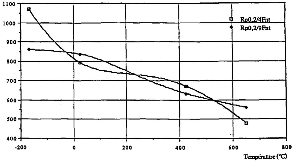
Figure 2 : Yield strenght evolution. Comparison between face 4F and 9F (non heat treated samples).
