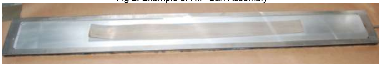
Fig 2. Example of HIP Can Assembly
