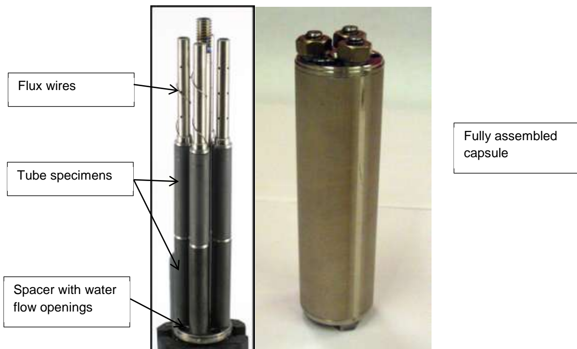
Figure 2. SiC/SiC tube sample fixturing. On the left is a partially assembled capsule showing tube samples positioned over the holder tubes and flux monitor wires. An assembled capsule is shown on the right with a flow shroud in place over the specimens between the top and bottom spacers.
