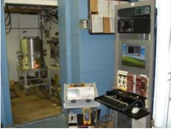
Fig 2. Conventional NDP setup at the RSEC neutron beam laboratory.
