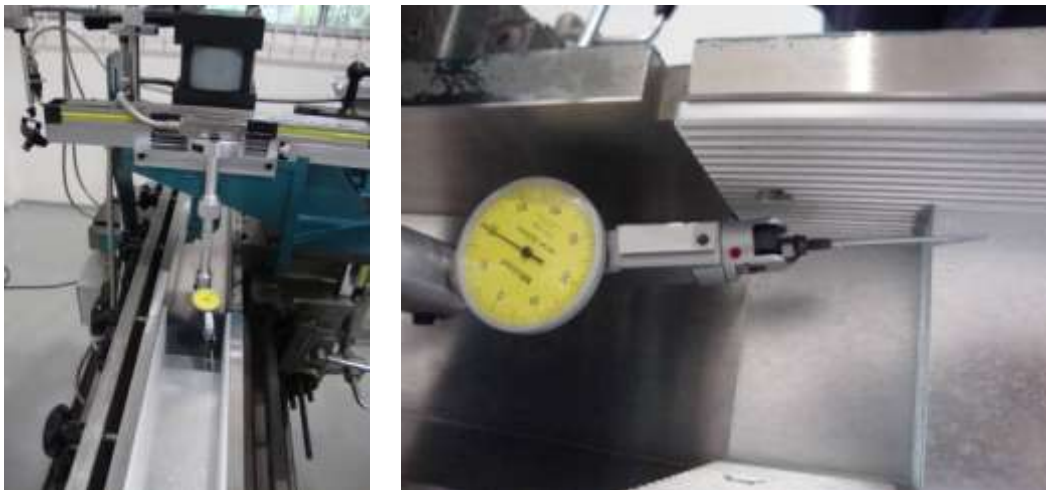
Fig 4 – Measurement system installed in the roll swaging machine
