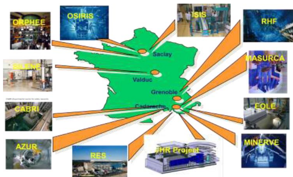
Fig. 1 Location of the French “fleet” of research reactors including OSIRIS/RJH: Materials testing reactor; EOLE/MINERVE : Mock-up in support to LWR studies; MASURCA: Mock-up in support to SFR studies; ISIS/AZUR/MINERVE: Education and training; ORPHEE/RHF: fundamental research reactor; CABRI/SILENE: Reactor for safety studies; RES : prototype reactor
