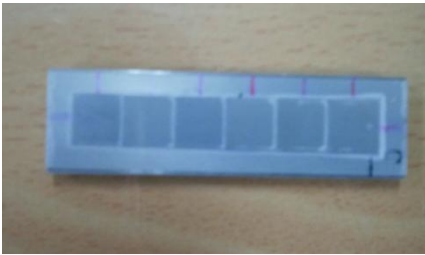
Fig. 3 Step wedge made of stainless steel foil
