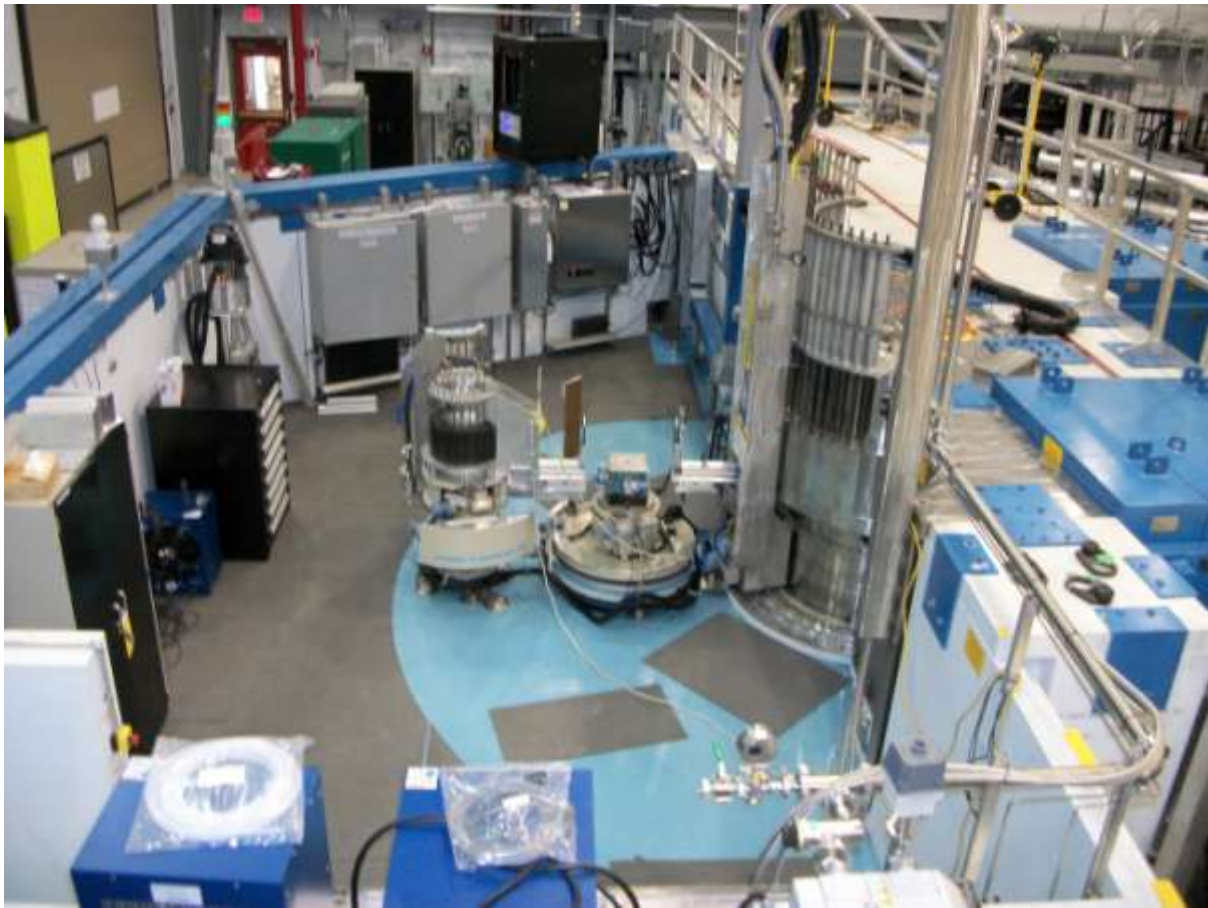
Figure 2: New Cold Triple Axis Spectrometer (CTAX) on Beam Line CG-4
