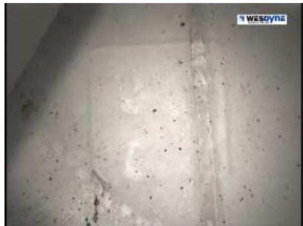
Fig 3. One of the bulges caused by the tank support leg pressure plates.
