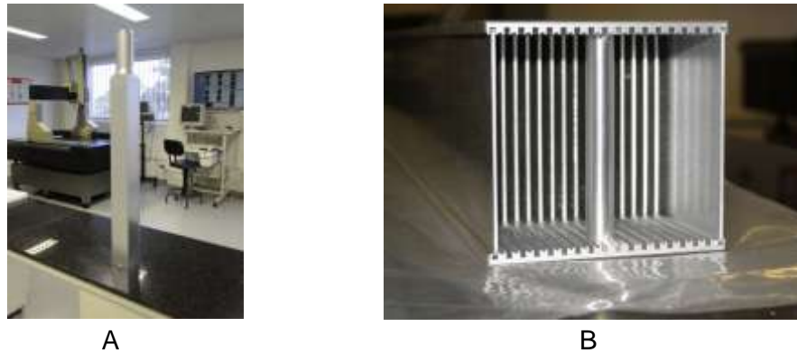
Fig 1 – Fuel element fabricated at IPEN (A) and details of the cooling channels (B)
