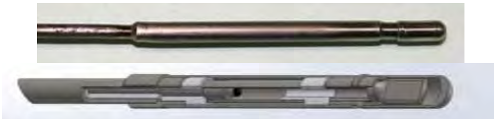
Figure 4. Picture and drawing of a 3 mm miniature gas ionization chamber manufactured by CEA
