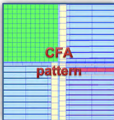
Fig 4. Pattern used for CFA cross section calculation (in red: Hf or water)
