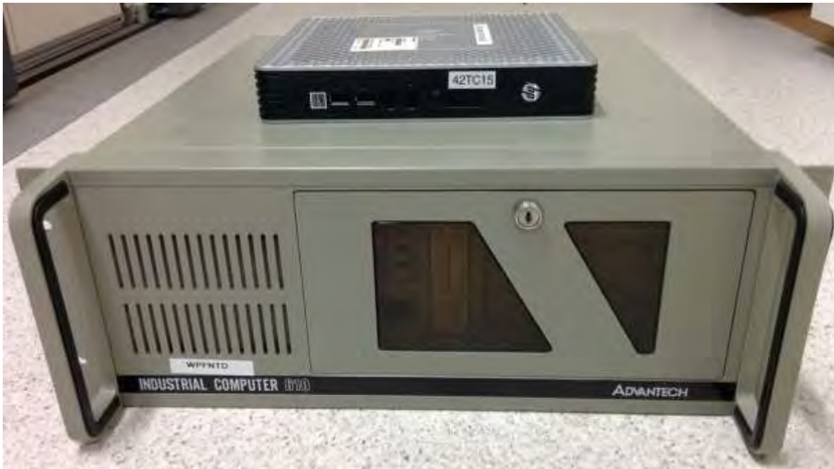
Fig 2. An operator workstation from the old system (bottom) with a new thin client (top).
