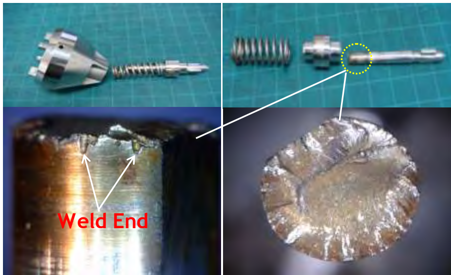
Figure 4. The failed rod tip of the capsule during the out-pile test
