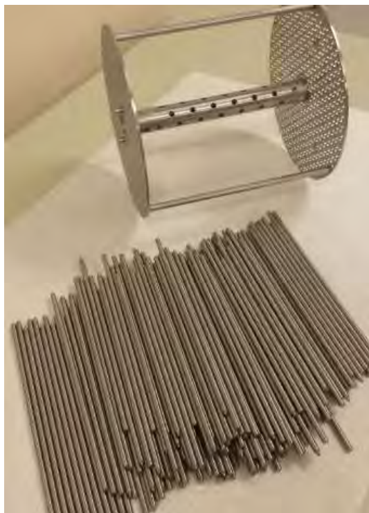
Figure 6 - Dummy LEU fuel cage with dummy fuel pins
