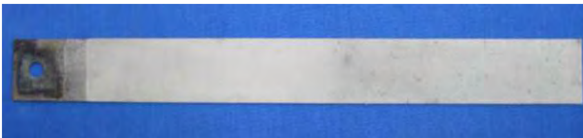
Figure 9 DU-10Mo foil acid etched in 8 molar nitric; residual salt removed with ethanol.
