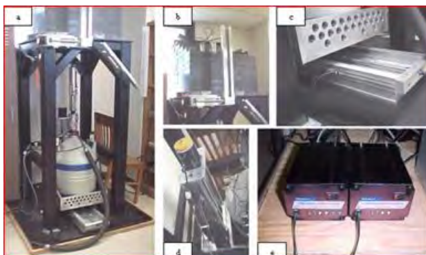
Fig 9. (a) Detector on transport (b) Sample loader (c) Horizontal slide (d) Vertical slide (e) Stepper motor controllers
