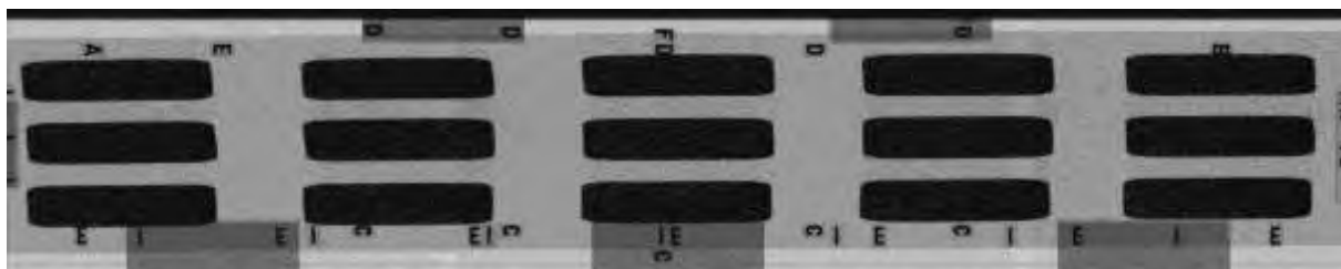
Fig 3. Mother plate containing multiple targets (15) after hot rolling
