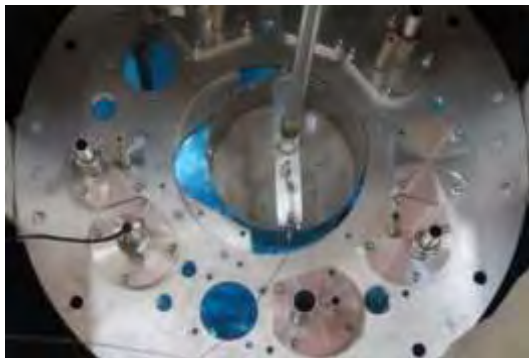
Figure 2 - Mock-up top plate with control rod support plate and shim tray
