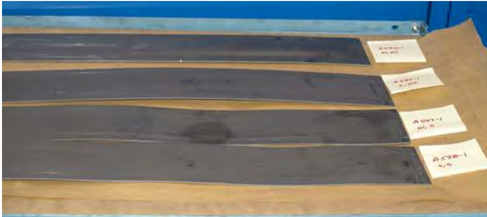
Figure 7: Fuel plates after HIP with the spring-loaded HIP.
