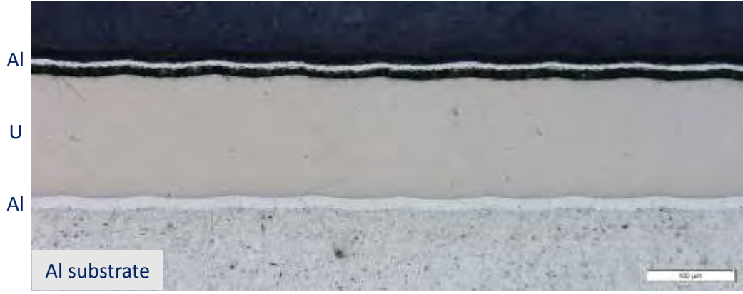
Figure 5: Microscopy of a sputtered Al-U-Al multilayer.
