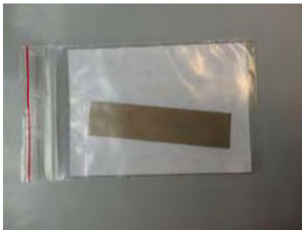
Figure 10: U-10wt.%Mo foil piece cleaned with SurTec 138 / SurTec 089 / H 2 O 2 solution under Ar atmosphere. No significant re-oxidation visible after one month.
