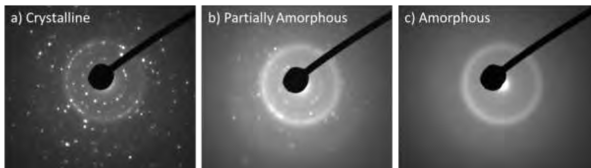
Fig 3. Evolution of the electron diffraction pattern from a) crystalline, to b) partially amorphous, and c) fully amorphous.
