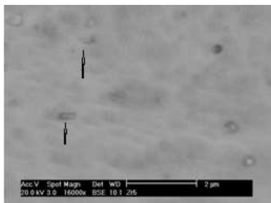
Fig 8. SEM analysis of the damaged peak region (located between 35 and 43 \mu\text{m} ) showing precipitates after 2.6 MeV proton irradiation to a fluence of 10^{17} p/cm 2 .
