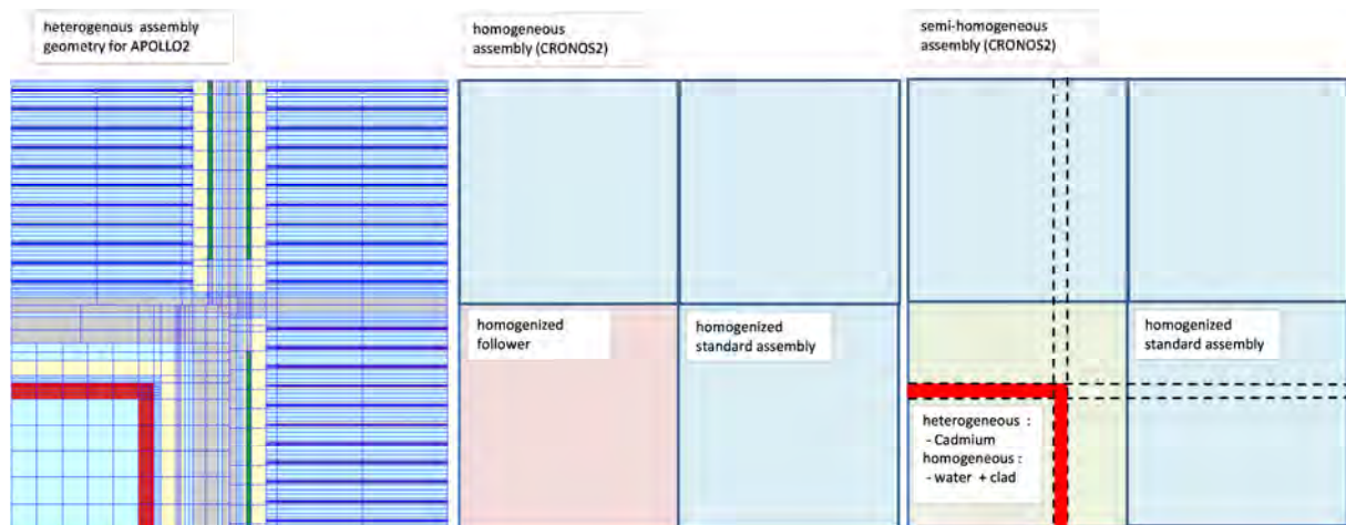
Fig 6 : Illustration of possible CRONOS2 meshes for follower-type control element. Exact geometry is left. Homogeneous 3D mesh is in the centre and semi-homogeneous is right. Calculation biases can be significantly reduced while only increasing CPU-time in a small proportion
