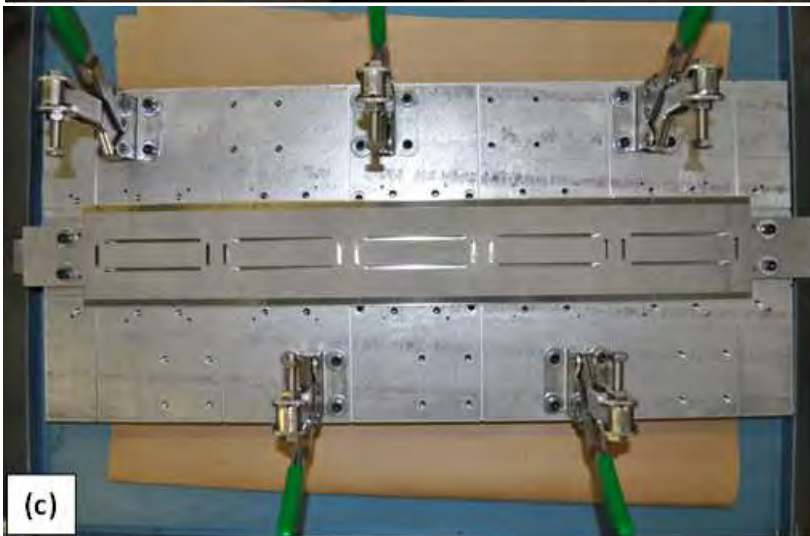
Figure 10: (a), (b) and (c): Steps in clamping sequence for producing MP-1 samples (shown outside of the EBW chamber).
