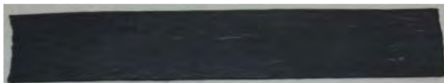
Fig 7. Assembly after hot rolling and uranium foil
