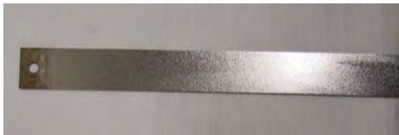
Figure 8 Du-10 Mo sample Electropolished for 10 min.
