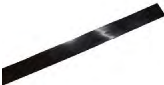
Figure 1: Oxidized DU-10wt.%Mo foil. Clearly visible is the thick black U oxide layer on the foil surface.
