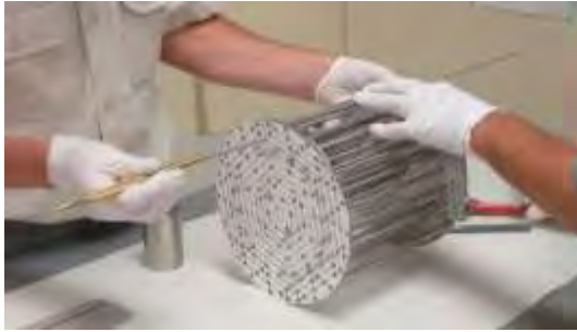
Figure 7 – Loading the dummy LEU pins into the dummy fuel cage and tolerances were tightened to keep the concentricity.
