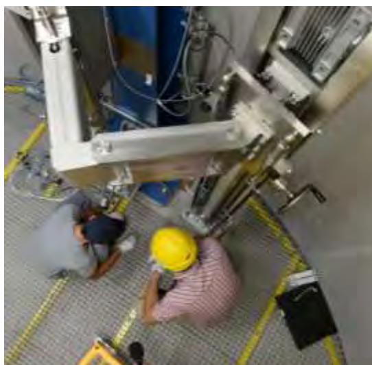
Figure 6 : articulated arm for actuators mounting on the hydraulic testing loop
