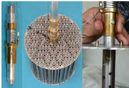
Figure 8 – Dummy LEU core and core lifting tool
