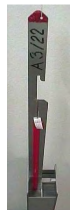
Fig 2. Copper wire on an aluminium blade
