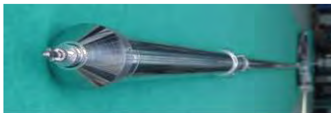
Figure 2. Standard material irradiation capsule at HANARO
