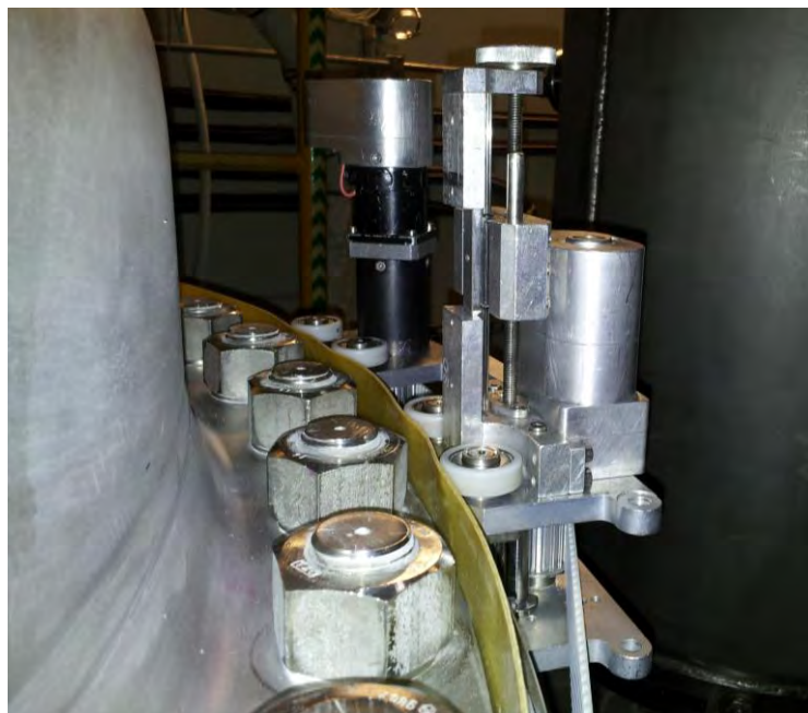
Fig. 3: UT generator and guiding system for mechanized ultrasonic tests (UT) of the primary heat exchanger.
